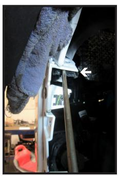
6. Unsnap the wheel well trim from the backside. Then insert a flat head screw driver between black and white pieces as shown and pull the fascia outward to remove. Do this on both sides of the vehicle.
