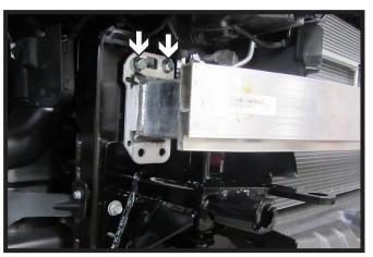
12. Reinstall bumper with spacer plate between the frame and the top of the bumper. Start the two (2) 10MM bolts with flat washers and lock washers. Do this on both sides of the vehicle
