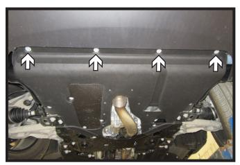
5. Using a 10MM socket, remove the four (4) bolts on the underside of the vehicle.
