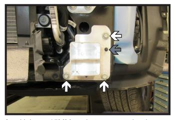
8. Using a 15MM socket, remove the three (3) bolts from the frame extension. Using a 10MM socket, remove the nut (gray) from the frame extension. Do this on both sides of the vehicle. The frame extension will not be reinstalled.
