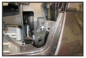
Using a T30 Torx, remove the two (2) bolts from the fascia, there is one (1) on each side.
