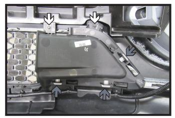
21. **Non-Shutter Models:** Using a 7MM socket, remove the two (2) bolts (white) from the air dam on the back side of the fascia. Unclip the three (3) clips (gray) by pushing down on the inside of the clip. Remove the air dam. Do this on both sides of the vehicle.
