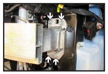
Using a 15MM socket, remove the four (4) bolts from the bumper. Using a 10MM socket, remove the nut (gray) from the bumper. Do this on both sides of the vehicle. Remove the bumper and set aside to be reinstalled later.
