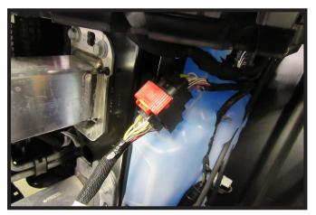
As the fascia is removed unhook the plug on the driver side by pulling out the yellow piece and up on the red part to unhook. Remove fascia and set aside to be reinstalled later.
