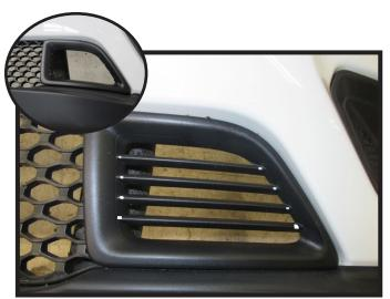
22a. **Non-Shutter Models:** Remove the horizontal slats from the corner of the fascia as shown. Do this on both sides of the vehicle.
