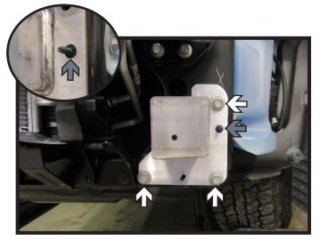
Using a 15MM socket, remove the three
