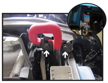
6. Using a 16MM socket, remove the two (2) bolts (white) from the underside of the tow hook. Using a 30MM socket, remove the nut (gray) from the backside of the tow hook (inset). Do this on both sides of the vehicle. Remove tow hooks and set aside, they will not be reinstalled.
