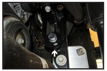
From the backside install the 1/2" x 5" bolt with lock washer and 1/4" x 2" DIA washer. Do this on both sides of the vehicle.
