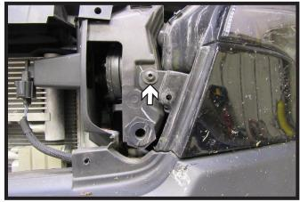
2. Using a T27 Torx, remover the one (1) screw from behind the fascia cover. Do this on both sides of the vehicle.
