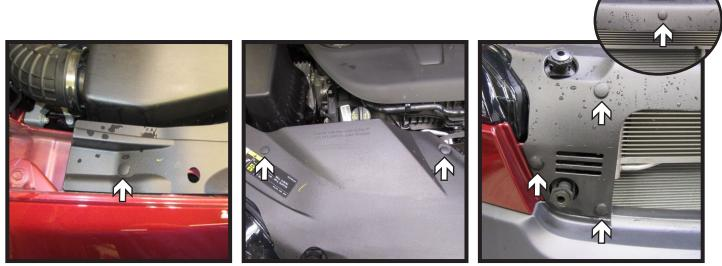
1. Remove the thirteen (13) push pins from the top edge of the fascia cover. There are six (6) on each side and one (1) in the center. Remove fascia cover and set aside to be reinstalled later.
