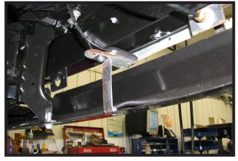
13. The breakaway bracket can be attached to the bottom edge of the bumper using a 1/4"-20 x 3/4" bolt with a 1/4"-20 nut. Trim the front cover (not shown) as needed to allow the breakaway to pass thru and attach the breakaway to the top of the bracket with a 1/4"-20 x 3/4" bolt and a 1/4"-20 nut.
