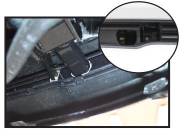
5. Temporarily reinstall the front cover. Hold the baseplate up as close to its installed position. Mark the backside of the front cover. Remove and trim the cover to allow the baseplate to pass thru. Do this on both sides of the vehicle.
