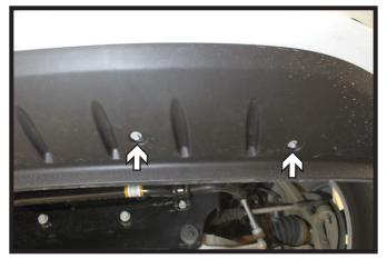
1. Using a 10MM socket, remove the four (4) screws from the front spoiler. There are two (2) on each side.
