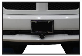
14. The electrical connection can be mounted in several locations with a combination of different hardware to suit the users need. Shown above is using the electrical bracket attached to the bottom of the license plate bracket.
