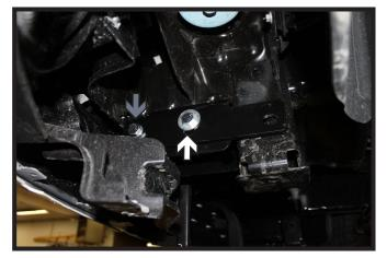
Bolt the side plate to the baseplate with a 1/2"-13 x 1-1/2" bolt with 1/2" lock washer and a 1/2"-13 lock nut into the front hole (gray) and a 1/2"-13 x 1-1/2" bolt with 1/2" lock and flat washers into the middle hole (white). Tighten all fasteners. Do this on both sides of the vehicle.
