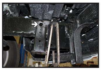
Clamp the baseplate into position. Using a 1-1/4" hole saw, drill an access hole above the tow hook bracket on the inside of the frame. Do this on both sides of the vehicle.
