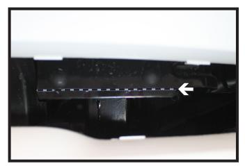
4. Using a reciprocating saw, trim the tow hook plates flush with the bottom of the bolts. Do this on both sides of the vehicle.
