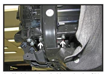
4. **Models equipped with tow hooks:** Slide the baseplate into position on the frame. Install two (2) 10MM-1.5 x 80MM bolts with 10MM lock washers into the bottom holes (white). Install 10MM-1.5 x 100MM bolts with 10MM lock and 3/8" flat washers through the baseplate into the bumper on both the front holes (gray). Tighten all hardware. Do this on both sides of the vehicle.
