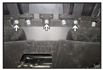
6. Using a 10MM socket, remove the three (3) center bolts from the front of the belly pan.
