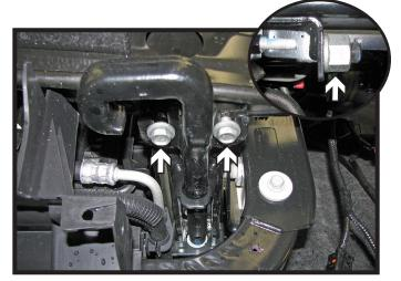
Models equipped with tow hooks: Using a 16MM socket, remove the two (2) bolts from the front side. Then using a 30MM socket or wrench, remove the nut from the backside of the tow hook. Remove the tow hook from the vehicle. Do this on both sides of the vehicle.
