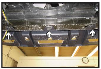
11. Turn the three (3) locking knobs on the bottom of the plastic shielding 90° to remove. Remove plastic shielding and set aside to be reinstalled later.
