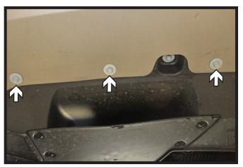
3. **Some Models**: Using a 10MM socket, remove the ten (10) bolts on the underside of the fascia. There are five (5) on each side of the vehicle.
