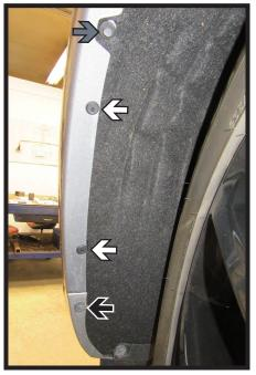
In the wheel well, using a 10MM socket, remove the top screw (gray). Using a 8MM socket, remove the lower screw (black). Then remove the two (2) plastic rivets (white). Do this on both sides of the vehicle.
