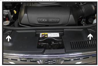
1. Remove the two (2) Phillips head push pins from the top edge of the fascia.
