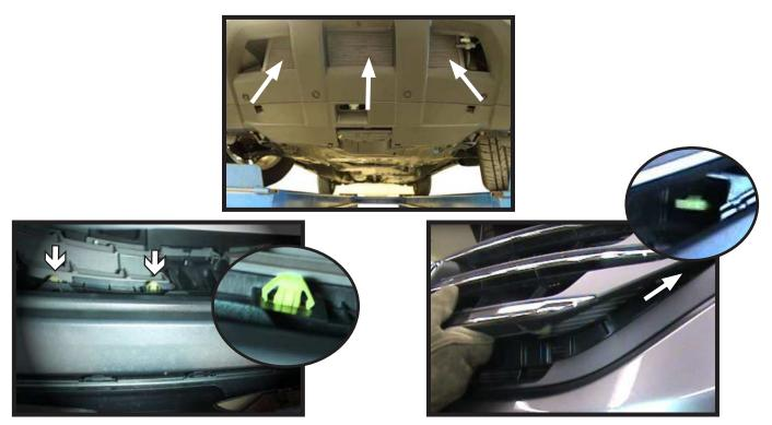
8. Looking from underneath the vehicle and toward the bumper, visually locate the four (4) yellow clips, two (2) on either side of the vehicle. From the front of the vehicle reach up into the openings and unhook these four (4) clips by releasing the top, bottom and sides of each clip, while maintaining slight outward pressure on top of the fascia.
