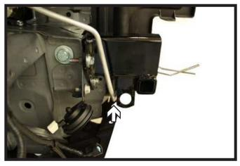
Make sure the coolant line does not interfere with the attachment tab. Then snap the coolant line back into the bracket.
