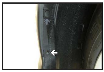
2. Using a Phillips screwdriver, remove the screw at the bottom of the wheel well (white). Then remove the two (2) push pins located above the screw (gray). Do this on both sides of the vehicle.
