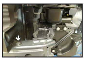
11. Using a flat screwdriver, remove the screw located on the top, outer edge of the bumper. Do this on both sides of the vehicle. The bumper will not be reinstalled.
