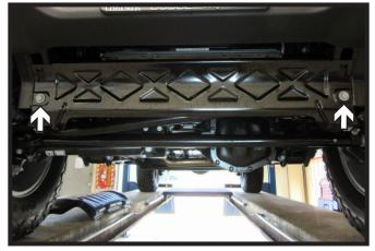
Sport, Sport S, & Overland Models: Using a 16MM socket, remove the two (2) bolts from the skid plate. Push up on skid plate to release clips and remove. Set aside skid plate to be reinstalled later.
