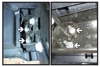
Using an 18MM socket, remove the four (4) nuts holding the bumper to the frame. Do this on both sides of the vehicle. Remove the bumper and set aside to be reinstalled later.
