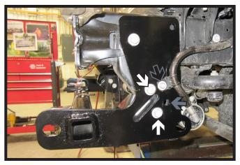
9a. Rubicon w/Steel Belly Pan Models: Place the belly pan bracket between the frame and the baseplate. Install the two (2) existing 10MM bolts (white). Then install the one (1) 1/2" bolt with hardware into the bottom back hole (gray). May need to ream out the bottom back hole.
