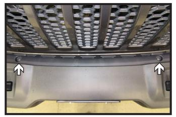
1. Remove the two (2) push pins, one (1) on each side, from the plastic piece behind the bumper.
