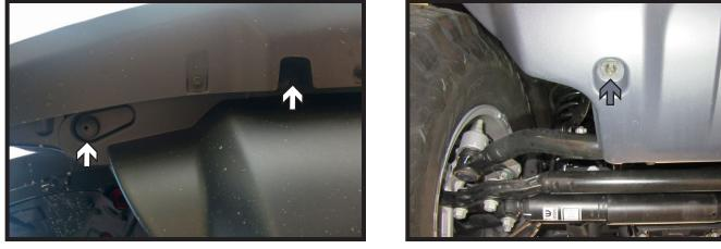
2d. **Overland Models:** Remove the nine (9) push pins from the front edge of the belly pan, there is one (1) in each corner and seven (7) along the center (white). Then using an 8MM socket, remove the two (2) bolts (gray), one (1) on each side, from the belly pan. Remove belly pan and set aside to be reinstalled later.
