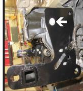
8. Hold frame bracket in place with vice grip (Left). Slide baseplate into position and start the top front 10MM existing bolt with hardware (Right). Ensure that all holes line up and the baseplate is level, then snug down bolt. Do this on both sides of the vehicle.
