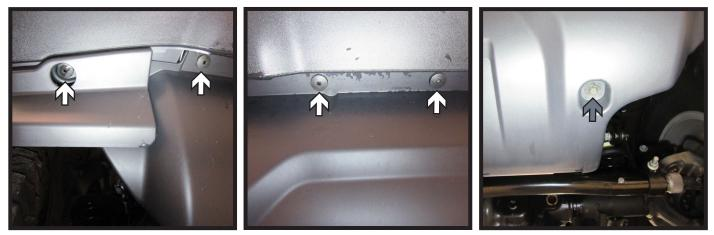
2c. **Sport & Sport S Models:** Remove the eight (8) push pins from the front edge of the belly pan, there are four (4) on each side (white). Then using an 8MM socket, remove the two (2) bolts (gray), one (1) on each side, from the belly pan. Remove belly pan and set aside to be reinstalled later.
