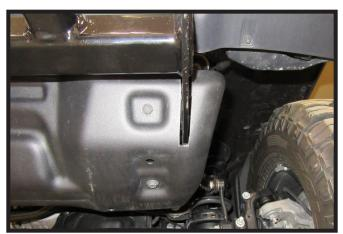
Trim belly pan for baseplate clearance in one of two ways listed below then reinstall belly pan.
