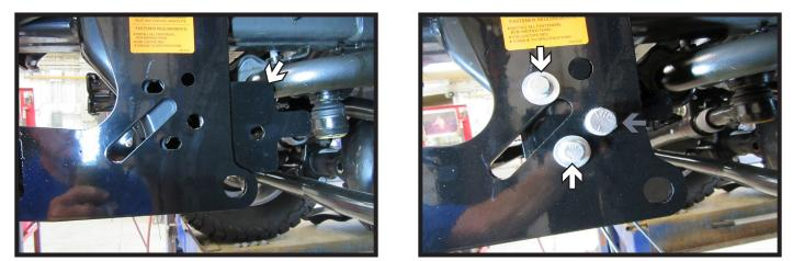
9b. **All Other Models:** Place the spacer plate between the frame and the baseplate. May need to use a pry bar to allow more room for the spacer plate to slide into place. Install the two (2) 3/8" bolts with hardware (white). Then install the one (1) 1/2" bolt with hardware into the bottom back hole. May need to ream out the bottom back hole. Do this on both sides of the vehicle.
