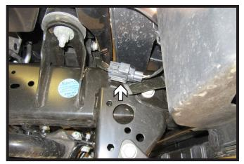
4. Unplug the indicated electrical from the passenger side of the vehicle.
