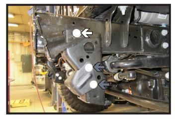
6a. **All Models:** Using a 16MM socket, remove the bolt holding the frame bracket (white).
