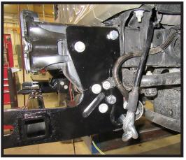
11. Attach the permanent baseplate safety cables to the provided convenience link on the baseplate. The photo above shows the recommended installation of the cables to frame of vehicle. Additional options may interfere with suggested mounting; in this case, secure the cables to a solid piece of the frame as described in the General Information sheet. Be sure the safety cables do not rub against any hoses or moving parts. Do this on **BOTH** sides of the vehicle.
