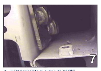
7. Hold baseplate to align with 17/32" drilled holes and insert the 1/2" nut plate, passenger's side into the frame end. Hand tighten the 1/2-13 x 1 1/2" hex bolts and the 1/2" lock washers. Do this to both sides of the vehicle. Reinstall metal bumper with existing metric bolts and clamp baseplate to the bottom of the metal bumper with the vise grips. Tighten 1/2-13 hex bolts with the 3/4" socket. Do this to both sides of the vehicle. **Be sure to apply LOCTITE Red to ALL bolts.**
