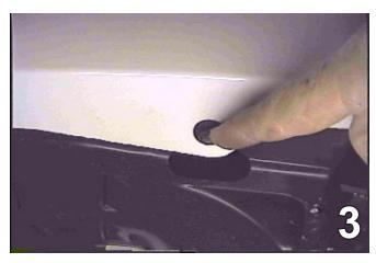
Using the 10MM socket, remove the metric bolts from the bottom edge of fascia. Do this to both sides of the vehicle. Set bolts aside to be reinstalled later.
