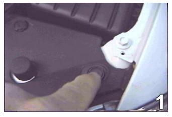
Remove ten pushpins from the top edge of the front fascia. Set pushpins aside to be reinstalled later.
