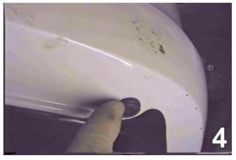
Remove four pushpins on the bottom side of the fascia. Pull fascia corners out to the side of the vehicle then forward to release. Set fascia and bolts aside to be reinstalled later.
