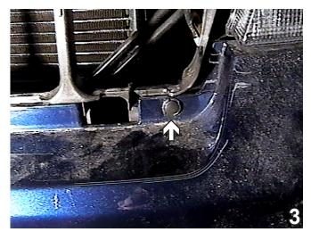
3. Remove four pushpins from the top edge of the metal bumper. Set the pushpins aside to be reinstalled later.
