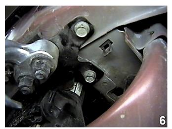
Using a 15MM socket, remove the factory tow hooks. Do this to both sides of the vehicle. The factory tow hooks will not be reinstalled later.
