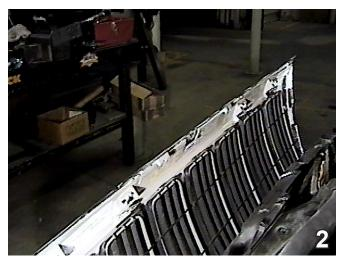
2. Pull the fascia forward and lift up to remove. Set the fascia aside to be reinstalled later.
