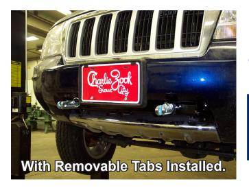
If the baseplate is in an accident, it must be replaced. DO NOT use it again! An accident can cause unseen damage and using it again could result in more damage or serious injury. DO NOT use the baseplate if it is damaged or missing parts.
