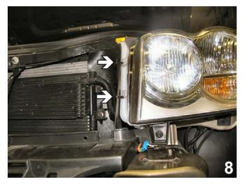
8. Remove two (2) christmas tree pushpins from the washer reservoir spout and air dam just inside of the headlight assembly on the driver's side.
