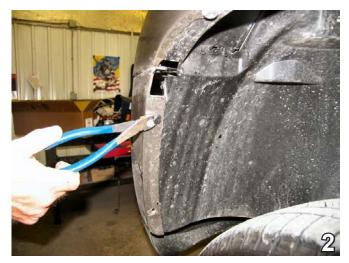
2. Using the diagonal cutters, remove two (2) rivets from the wheel well cover just forward of the front tires. Do this to both sides of the vehicle. These rivets will be replaced.
