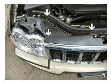
Remove the six (6) pushpins from the black plastic cover on the top side of the fascia. Lift cover up and set aside to be reinstalled later. Pull top of grille forward. Lift up and set aside with pushpins to be reinstalled later.
