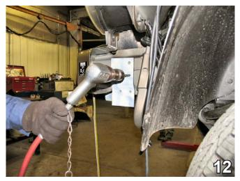
12. Using the baseplate as a template, drill **ALL** holes with the 13/32" drill bit. Do this to both sides of the vehicle.
