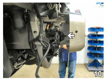
10. Remove the metric bolt from the horn bracket on the passenger's side with the 13MM socket, unplug the electrical and set horn assembly aside.
