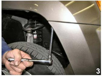
3. Using a 7MM socket, remove one (1) metric bolt from just forward of the front tire, on the fascia's corner. Do this to both sides of the vehicle. Set the bolts aside to be reinstalled later.
