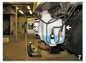
Using the 10MM socket, remove two (2) metric bolts from the washer reservoir on driver's side, unplug the electrical connections, disconnect and plug fluid lines. Set bolts aside to be reinstalled later
