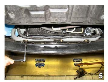
5. Using the 10MM socket, remove three (3) metric bolts from the lower radiator cross member. Pull the fascia forward, unplug the electrical connections. Set the fascia and the bolts aside carefully to be reinstalled later.
