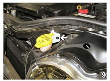
9. Remove a rivet from the reservoir spout with the diagonal cutters, pull reservoir down and set aside to be reinstalled later.
