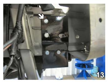
Insert the two (2) nut plates into the end of the frame rail to align with the top two (2) drilled holes, tighten the 3/8"-16 hex bolt and lock washer with the 9/16" socket. Do this to both sides of the vehicle.
