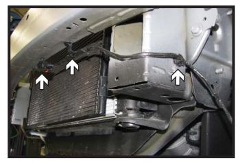
Disconnect the temperature sensor from the underside of the bumper/frame and set aside.
