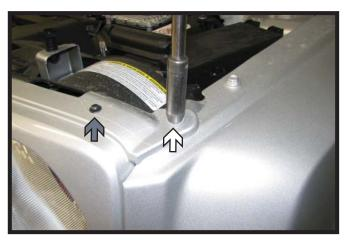
Using a 10MM socket, remove the two (2) screws from the top corner of the fascia.
