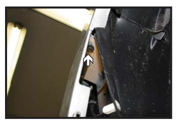
Pull back the wheel well liner, then using a 7MM socket, remove the screw from the fascia/fender joint. Do this on both sides of the vehicle.
