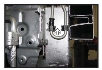
11. On the passenger side, if necessary, slide the coolant tube up out of the way and move the stoppers down to hold it.
