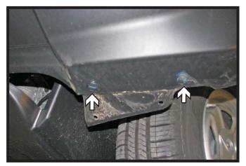
4. Remove the four (4) push pins from the underside of the fascia. There are two (2) on each side.
