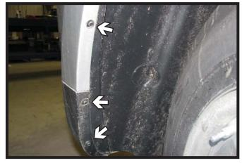
Using a 7MM socket, remove the three (3) screws from along the edge of the wheel well. Do this on both sides of the vehicle.
