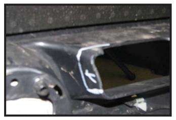
19. Hold the fascia up to the vehicle and trim the plastic intake slots as needed to clear the baseplate.
