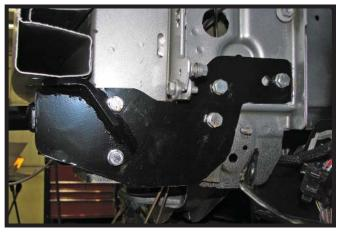
14. Continue drilling the remaining holes thru the frame and installing the appropriate hardware/spacers as needed. Do this on both sides of the vehicle. Fully tighten all hardware.
