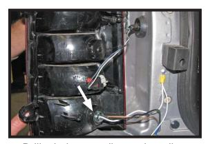
Drill a hole according to the tail light wiring kit instructions.
