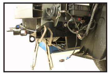
6. Slide the baseplate onto the vehicle. Level and clamp the baseplate to the frame.
