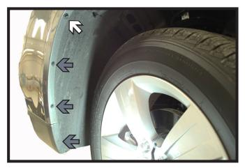
3. Using a 10mm socket, remove the top screw from the wheel well (white). Then using a 7MM socket, remove the other three (3) screws (gray).
