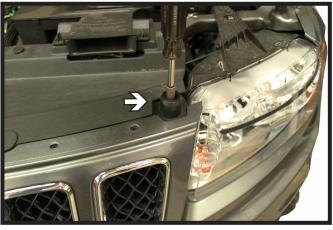
2. With a 27 Torx remove the two (2) bolts that are located on the upper side of the vehicle, one (1) per side.
