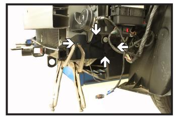
7. Using a 13/32" drill bit, drill the four (4) holes in the baseplate thru the frame. Install 3/8"-16 x 1-1/2" bolts with 3/8" lock washers into the holes and 3/8" nut plates on the inside of the frame. Do this on both sides of the vehicle. Fully tighten all hardware.
