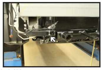
5. On the passenger side, remove the push pins that hold the temperature sensor in place. Gently set it over to the side of the vehicle until after the baseplate has been installed. Once the baseplate has been installed, put the push pins on the side and front back to the original location. Using a cable tie, secure the temperature sensor to the baseplate.
