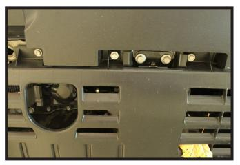
4. Using a 10MM socket, remove the three bolts from the underside of the fascia. There are two (2) towards the center and one (1) towards the passenger side.
