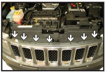
1. Using a T20 Torx, remove the seven (7) screws from the top edge of the fascia. There are four (4) on the passenger side and three (3) on the driver side.
