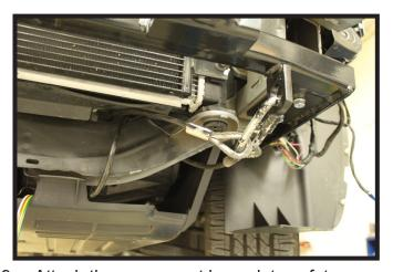
9. Attach the permanent baseplate safety cables to the provided convenience link on the baseplate. The photo above shows the recommended installation of the cables to frame of vehicle. Additional options may interfere with suggested mounting; in this case, secure the cables to a solid piece of the frame as described in the instructions included with the permanent baseplate safety cables. Be sure the safety cables do not rub against any hoses or moving parts. Do this on BOTH sides of the vehicle.
