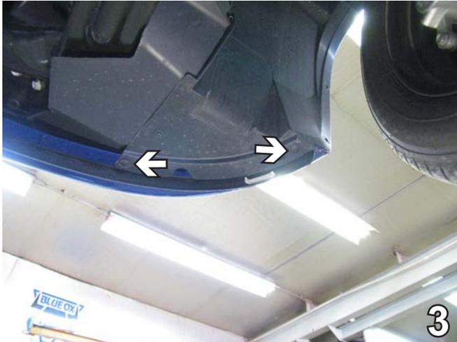
3. Just forward of the front tires, on the under side of the front fascia, remove two push pins. This is done on both sides of the vehicle, the passenger's side is shown. Set the push pins aside to be reinstalled later. Pull fascia forward and carefully set aside to be reinstalled later.
