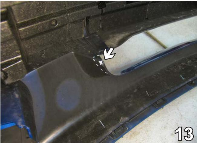
13. On the back side of the fascia, use a utility knife to trim 3/4"-1" from the outside edge of the opening to allow the attachment tabs to come through. Some models may not require cutting. Try to put fascia on and check to see if trimming is necessary.
