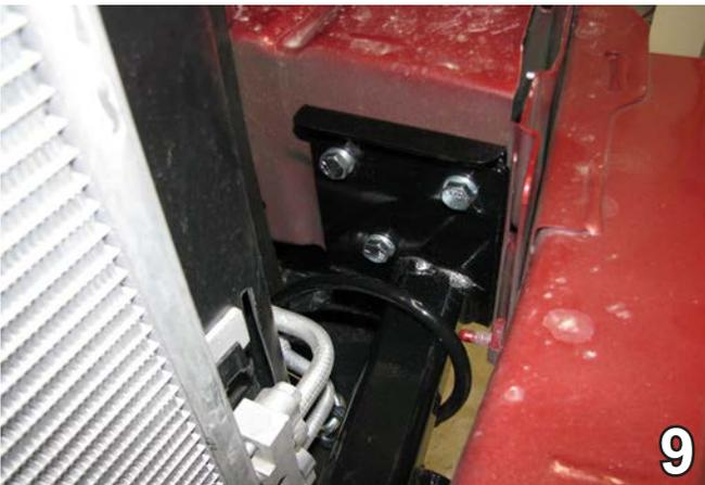
9. Insert the three 3/8-16 nut plates into the top of the frame rail and install the three 3/8-16 x 1 1/2" hex bolts and 3/8 Lock Washers. Cut the excess wire from the nut plates once they are installed. This is done on both sides of the vehicle, the driver's side is shown.
