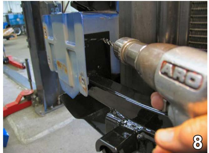
8. Using the baseplate as a template, drill the two front holes in the end plates with the 13/32" drill bit. To prevent drilling into the radiator, place something between the drill and the radiator and drill the back hole at an angle. This is done on both sides of the vehicle, the passenger's side is shown.
