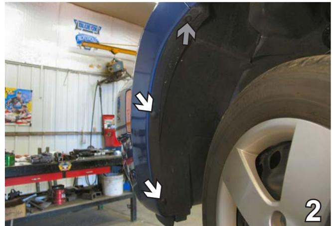
2. Just forward of the front tire, remove one 7MM bolt with the 7MM Socket (see grey arrow) and remove two push pins (see white arrows). This is done on both sides of the vehicle, the driver's side is shown. Set all aside to be reinstalled later.
