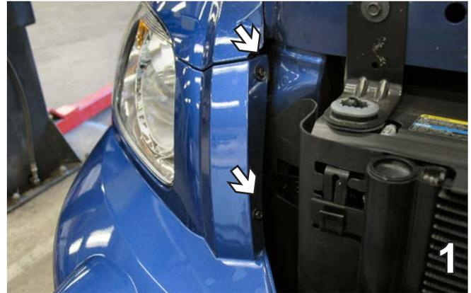
1. Using the 7MM Socket remove two 7MM bolts from the front fascia near the headlight housing. This will need to be done to both sides of the vehicle, the passenger's side is shown. Set bolts aside to be reinstalled later.
