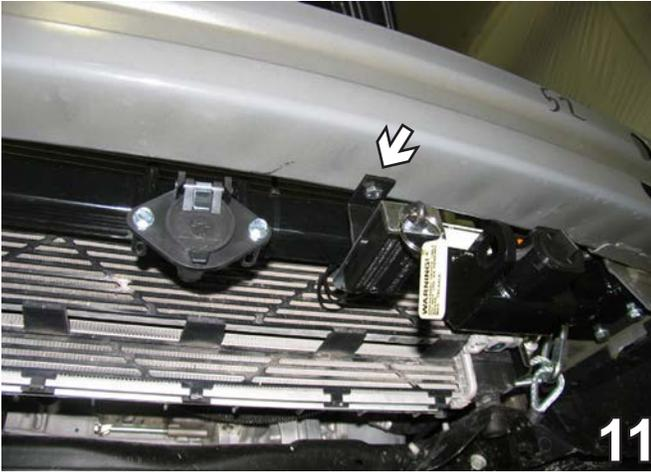
11. To install breakaway bracket, drill into the bottom of the bumper, centered between the electrical plug and the convenient link.
