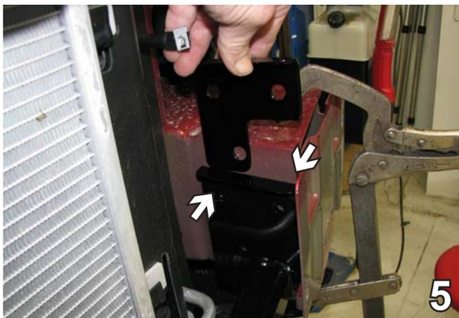
5. From the bottom of the vehicle, slide the baseplate up inside the frame rail until the bottom end plates are flush with the bottom of the frame rail, center and clamp. If needed tap the proper plate in behind the baseplate on each side.
