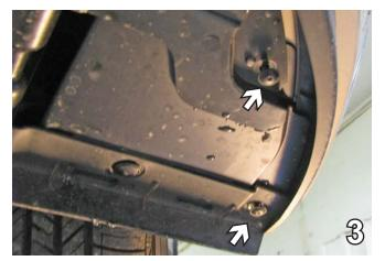
3. Remove the two (2) bolts from underneath the fascia, just forward of front tires with the T20 Torx, both sides. Set the bolts aside to be reinstalled later.
