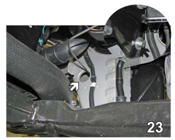
23. Insert 3/8"-16 x 1-1/2" hex bolt with 3/8" lock washer into the lower inside hole on the baseplate (black arrow step 22). Fasten to a 3/8" nut plate inserted through an existing hole underneath in the frame (white arrow). Do this on both sides. Be sure to use Loctite Red on the bolts.
