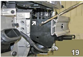
19. Slide the baseplate onto the frame rail flush with the top and as far forward as possible. Be sure support plate holes are in line with the existing holes (step 21). Then clamp the baseplate to the frame rail with the large vise grip.
