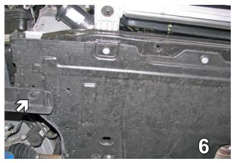
6. Remove one (1) push pin from the bottom of the belly pan. Do this on both sides. Set push pins aside to be reinstalled later.
