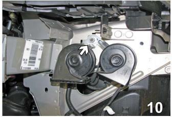
10. Using the 13MM socket, remove the metric bolt from the horn bracket on the driver side, unplug and set the bolt and horn aside to be reinstalled later.
