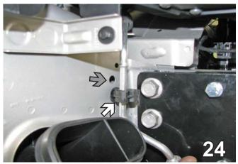
24. On the passenger side in the corner next to the baseplate, drill a 1/4" hole below the large hole (gray arrow) and pop the clip back in (white arrow). Be sure it is low enough so that the line clears the baseplate. Reattach the horn bracket on the driver's side. Reattach the air intake tube and the belly pan.
