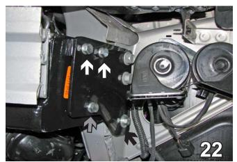
22. Bolt the upper two (2) holes (white arrows) with 3/8"-16 x 2" hex bolts, 3/8" lock washers and fasten to 3/8" nut plates inserted through the drilled hole in the bumper. In the lower outside hole (gray arrow) bolt the support plate to the baseplate with 3/8"-16 x 1-1/2" hex bolt fastened with 3/8" lock washer and 3/8"-16 hex nut. Be sure to use Loctite Red on all bolts. Do this on both sides.
