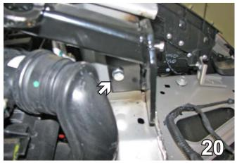
20. Using the baseplate as a template, drill a hole on the bottom side with the 13/32" drill bit. Insert 3/8"-16 x 1-1/2" hex bolt with Loctite Red and 3/8" lock washer. Attach to 3/8" nut plate inserted through the 1-1/2" lower opening on bumper. Do this to both sides.
