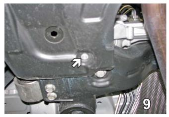
9. Using an 8MM socket, remove one (1) more metric bolt toward the back of the belly pan. Do this on both sides. Set bolts aside to be reinstalled later.
