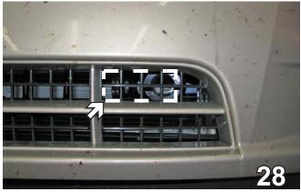
28. Hold fascia up to its original position. Using the diagonal cutters, cut out the upper outside area of the front fascia allowing room for the attachment tabs to come through the grille. Do this on both sides. Reinstall the fascia.
