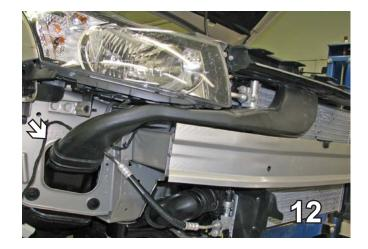
12. On the passenger side below the headlight, detach the air intake tube from the bottom section of the tube. Set aside to be reinstalled later.
