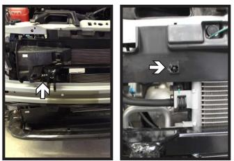
12. Trim the passenger side baffle around the baseplate and reinstall. Reinstall the temperature sensor into the baffle (right).
