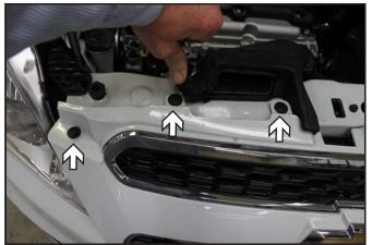
1. Remove the six (6) push pins from along the top edge of the fascia. There are three (3) on each side.
