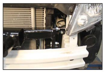
Install the baseplate onto both end plates, using the 3/8" hardware. Fully tighten down the baseplate and end plate bolts.
