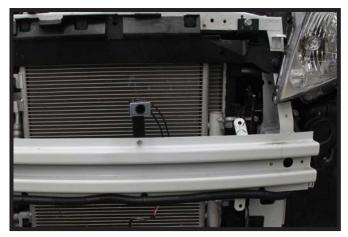
Optional Breakaway: Install the bracket to the bumper with the 1/4" hardware approximately 16" from the end on the driver side or in the desired location.
