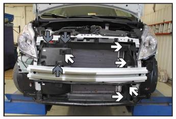
5. Remove the four (4) push pins from the driver side air baffle (white) and set it aside. Then remove the three (3) push pins (gray) and temperature sensor (white) from the passenger side air baffle and remove the baffle from vehicle.
