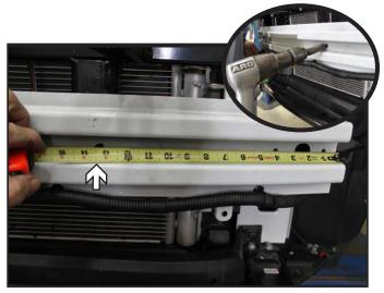
10. Using a 3/8" drill bit, drill a hole thru the bumper 13-1/2" in from the end. Repeat on the other side of the vehicle.
