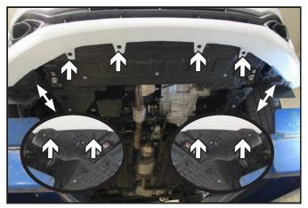
Using a phillips screwdriver or 7MM socket, remove the eight (8) screws from the bottom edge of the fascia. There are four (4) on each side of the vehicle.
