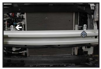
7. Bend the passenger side bumper tab back slightly for baseplate clearance (white).
