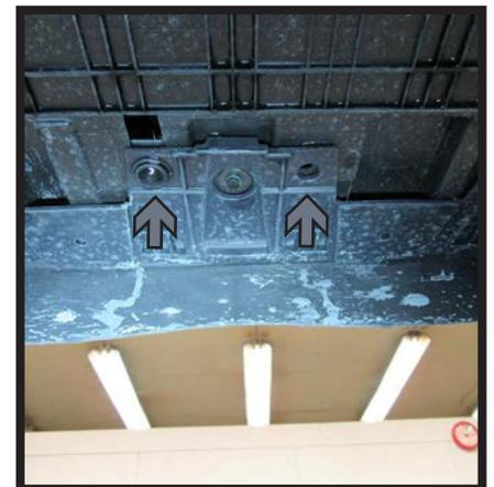
3. Using a 7MM socket, remove the six (6) bolts (white) from the underside of the vehicle. There are three (3) on each side of the car. Remove the two (2) push pin (gray) from the center of the underside.
