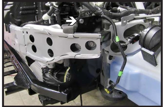
8. Slide the baseplate into position and ensure it is level, then slide spacer plate into position between frame and baseplate before clamping to the frame rail on both sides with large vise grips.
