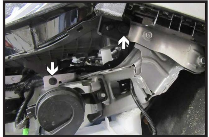
6. Using a 7MM socket, remove the four (4) bolts from the headlight. There are two (2) on top of the headlight area, and two (2) below the headlight on the side. Remove the headlight and set aside. Do this for both sides of the vehicle.
