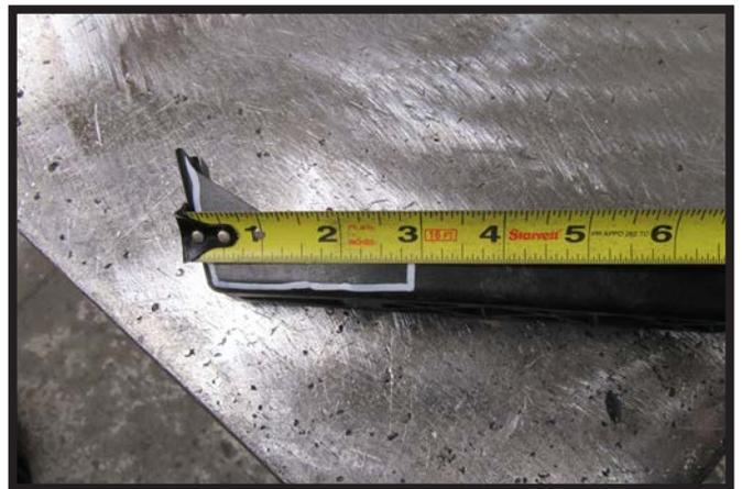
12. Before reattaching the front brace. Mark brace 3" from bottom corner then down and across as indicated. Do this for both sides of the brace. Then using a reciprocating saw trim marked area to allow the brace to sit further back on the baseplate when reattached.
