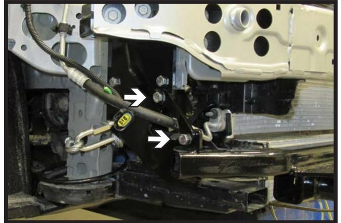
10. On the passenger side, attach the flat plate with the provided 3/8" hardware.
