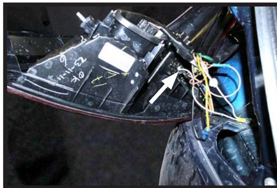
Drill a hole according to the tail
