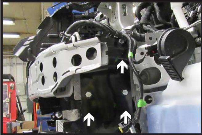
9. Using a 3/8" drill bit, drill out the remaining three (3) holes and insert the provided 3/8" hardware. Do this for both sides of the vehicle.
