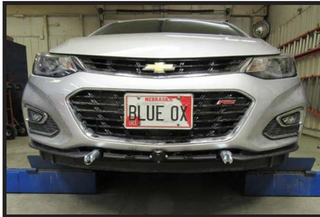
13. Hold the fascia as close to its original position, mark and trim the fascia around the convenience links and attachment tabs. Reinstall the center brace, headlights, fascia and fascia cover.
