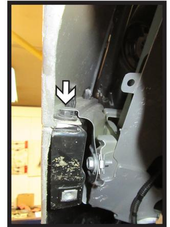
2. Using a T15 Torx, remove the two screws from the edge of the wheel well in front of the tire. Next, pull the cover back. Using a 7MM socket, remove the one (1) bolt from under the cover. Do this for both sides of the vehicle.
