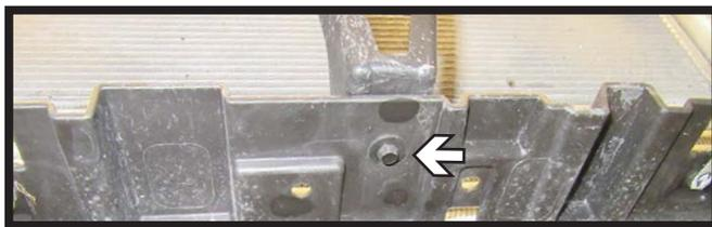
7. Using a 7MM socket, remove the two (2) bolts from the brace on the front of the fascia. One (1) from the top and one (1) from the bottom of the brace.
