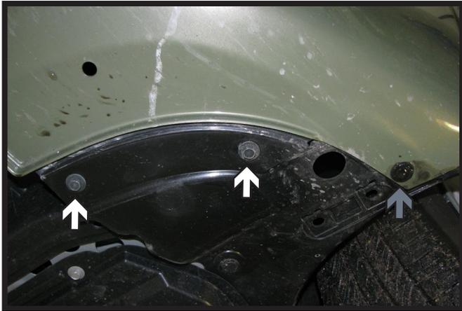
5. Using a 10MM socket, remove the two (2) screws from underside of the fascia (white). Then remove the outer push pin (gray). Do this on both sides of the vehicle.
