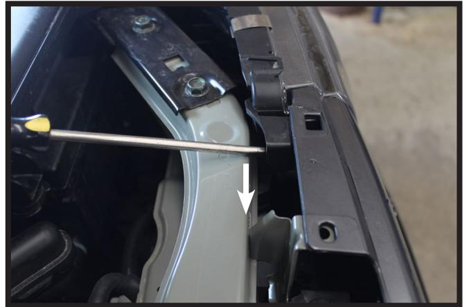
2. Using a flat screwdriver, release the clip towards the driver side.
