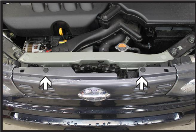
1. Remove the two (2) push pins from the top edge of the fascia.
