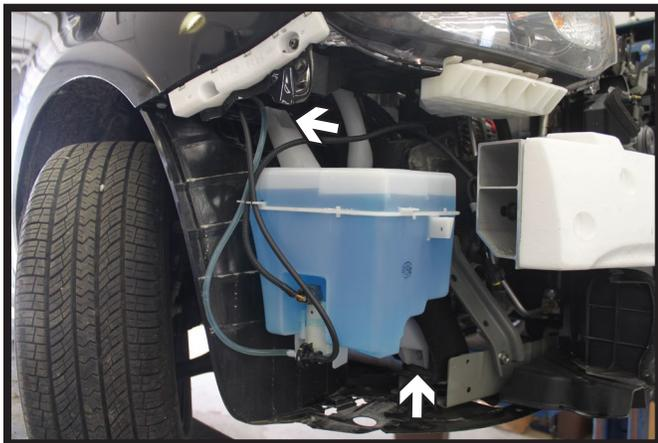
7. Using a 10MM socket, remove the two (2) screws from the washer reservoir. Disconnect/Plug all lines, separate the reservoir from the filler tube and set aside.
