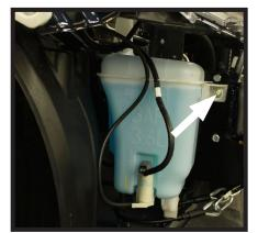
Reconnect the windshield wiper fluid reservoir using the existing fasteners except for the top, front hole. For this, use the 6MM-1.0 x 30MM hex head bolt and the 1/4" washer that has been provided.
