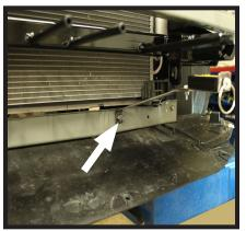
9. Using the existing stud, attach the breakaway bracket and securely fasten with the 8MM x 1.25 nut that has been provided.
