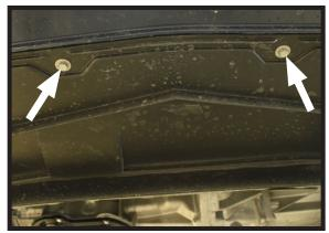
3. Remove the two (2) 10MM bolts that are located in the center.
