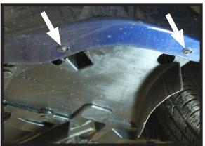
2. Using a T20 Torx remove the two (2) screws underneath the vehicle on the outside edge. Towards the center there are three (3) push pins that need to be removed. Do this on **BOTH** sides of the vehicle.
