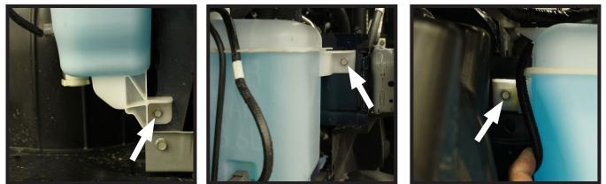
6. With a 10MM socket remove the three (3) bolts that hold the windshield wiper fluid reservoir in place. On the front of the reservoir there is one (1) bolt at the bottom and one (1) towards the top. On the backside of the reservoir is the 3rd bolt. It may be necessary to push back on the wheel well liner to access this bolt.
