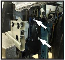
8. Slide the baseplate downward at a slight angle and then up so the baseplate frame runs parallel with the vehicle's main frame. The top of the baseplate end plate should be flush with the top of frame. The back edge of the baseplate end plate should be aligned with the front edge of the main frame.
