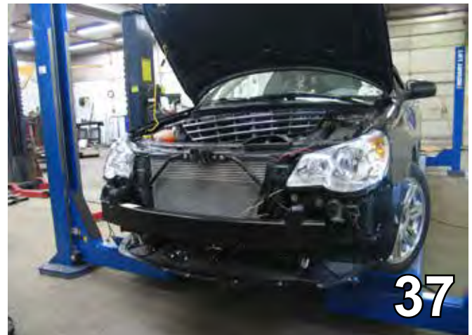
37. Reinstall the headlight assembly, reconnect the transmission coolant line, reconnect the sensor, replug the running lights, reinstall the fascia and the grille.
