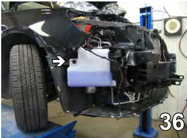
36. Reinstall coolant line brace from step 22 with a 6MM-1.00 x 30MM bolt, 6MM lock washer and a 1/2" spacer. Then reattach the washer reservoir and reconnect the hoses and electrical connections with existing hardware.
