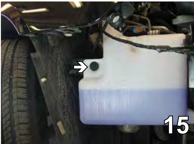
15. Using a 10MM socket, remove the bolt on the outside of the washer reservoir. You will then need to unplug the hoses and electrical connections. Set the bolts and washer reservoir aside to be reinstalled later.
