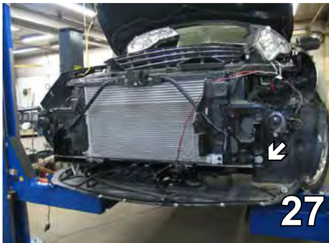
27. Measure out 3 3/8" just below the lower bumper from the bolt to the front edge of the baseplate on both sides. Be sure the baseplate is level across the top and clamp.
