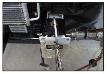
Drill the top front hole thru frame using a 13/32" drill bit. DO NOT drill remaining holes at this time.
