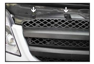
On top of the grill locate and remove the two (2) screws using a 25 Torx. Do this on both sides of vehicle. After the four (4) screws are removed the grill can be removed from the vehicle.
