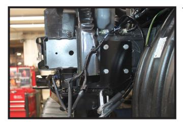
15. Attach the permanent baseplate safety cables to the provided convenience link on the baseplate. The photo shows the recommended installation of the cables to frame of vehicle. Additional options may interfere with suggested mounting; in this case, secure the cables to a solid piece of the frame as described in the instructions included with the permanent baseplate safety cables. Be sure the safety cables do not rub against any hoses or moving parts. Do this on **BOTH** sides of the vehicle.
