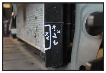
On the driver side, just below the rib, make a 1/2" deep x 2" high notch in the plastic shrouding for baseplate clearance.
