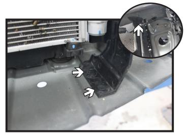
7. Remove the three (3) push pins from the plastic shielding next to the radiator. There are two (2) the bottom and one (1) just under the bumper. Do this on both sides of the vehicle. The shielding will not be reinstalled.
