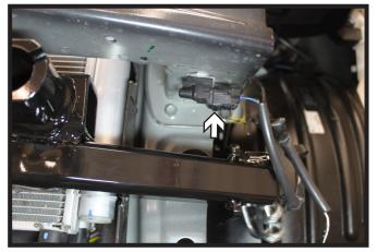
16. Reinstall the temperature sensor on the underside of the bumper.
