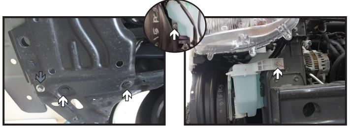
5. Using a 12MM socket, remove the screw from the underside of the vehicle on the passenger side (gray). Then remove the two push pins next to the screw.
