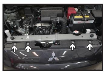
1. Using a 10MM socket, remove the four (4) screws from the top edge of the fascia.
