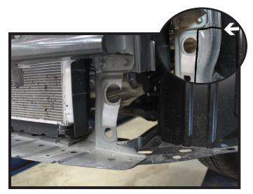
9. Using a reciprocating saw, trim the frame face just below the bumper along the edge of the hole down to the base. Do this on both sides of the vehicle.
