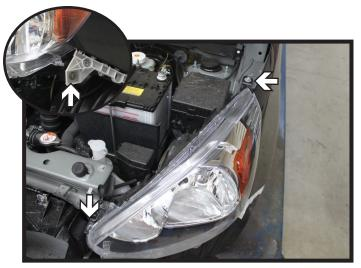
Using a 10MM socket, remove the three
