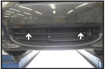
4. Using a 10MM socket, remove the two (2) screws from the front of the fascia.
