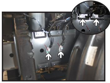
8. Using a 10MM socket, remove the two (2) ground straps from the driver side.
