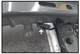
6. Remove the temperature sensor from the underside of the bumper on the driver side and set aside until after baseplate installation.
