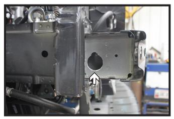
10. Using a 1-1/4" hole saw, drill an access hole on the passenger side bumper as shown for nut plate access.
