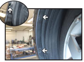
2. Remove the three (3) push pins from the wheel well. There are two (2) on along the lower edge and one (1) above. Do this on both sides of the vehicle.
