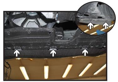
3. Remove the seven (7) push pins from the underside of the fascia. There are two (2) on each side and three (3) in the middle.
