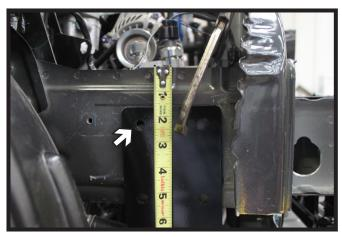
Position the baseplate onto the vehicle. Measure down an 1-5/8" from the top of the frame and allow about a 1/4" of clearance around the coolant line in front.
