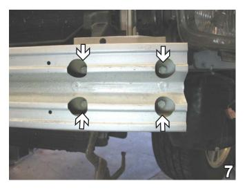
Using the 13mm socket, remove four metric bolts from the metal bumper. Do this to both sides of the vehicle. Pull metal bumper forward to remove. Set bolts and metal bumper aside to be reinstalled later.
