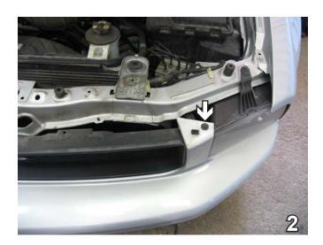
2. Using the 10mm socket, remove one metric bolt from the top of fascia, next to the headlight assembly. Do this to both sides of the vehicle. Set bolts aside to be reinstalled later.
