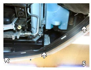
Remove seven Phillips pushpins along the bottom of fascia, three each side and one in the center. Pull fascia forward to remove. Set pushpins and fascia aside to be reinstalled later. Passenger's side is shown.
