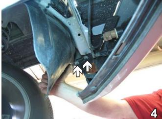
Push wheel well cover aside to remove two metric bolts and nuts from the upper corner of fascia using the 10MM socket. Do this to both sides of the vehicle. Set bolts aside to be reinstalled later.
