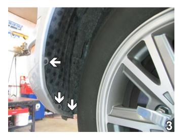
Just forward of the front tire, on edge of fascia, remove three Phillips screws. Do this to both sides of the vehicle. Set screws aside to be reinstalled later.
