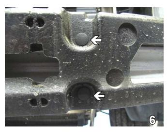
6. Remove two Christmas tree pushpins from front of styrofoam bumper. Do this to both sides of the vehicle. Pull styrofoam bumper forward to remove. Set styrofoam bumper and pushpins aside to be reinstalled later.
