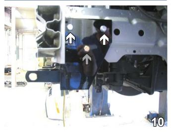
10. Using baseplate as a template, drill 3 holes in frame rail with the 13/32" Carbide drill bit. Insert 3/8-16 nut plates into opening of frame rail and align with upper two holes. Insert 3/8-16 x 1 1/2" bolts and 3/8" lock washers into upper two holes and tighten to 3/8-16" nut plates (see white arrows). Install 3/8-16 x 1 3/4" bolt, 3/8" spacer pipe, 3/8" lock washer and 3/8-16 hex nut to lower hole (see grey arrow). Do this to both sides of the vehicle.
