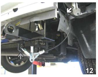
12. Attach the permanent baseplate safety cables to the provided convenience link on the baseplate (see grey arrow). The photo above shows the recommended installation of the cables to frame of vehicle (see white arrow). Additional options may interfere with suggested mounting; in this case secure the cables to a solid piece of the frame as described in the instructions included with the permanent baseplate safety cables. Be sure the safety cables do not rub against any hoses or moving parts.
