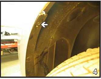
4. Using 6MM socket, remove one (1) screw from edge of fascia, just inside the wheel well. Do this to both sides of the vehicle. Set screws aside to be reinstalled later.
