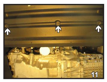
11. Using the flat screwdriver, remove three (3) push pins on the bottom and remove the black plastic piece. Set push pins and plastic aside to be reinstalled later.
