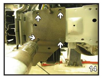
14. Using the baseplate as a template, drill four (4) corner holes into the frame webbing with the 13/32" drill bit. Insert 3/8"-16 x 1-1/4" hex bolts into holes and tighten to the 1/4" lock washers and 3/8"-16 hex nuts.
