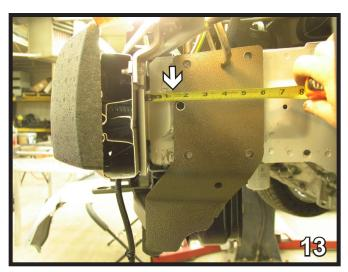
13. Slide the baseplate onto the frame rails 1- 1/2" back from the bumper bracket aligning the front air baffle hole with the front middle hole of the baseplate. Align the top edge of the endplate with the top edge of the frame rail and clamp in place using the large vise grips. Hold the fascia up to its original position and verify the convenience links, electrical rods and attachment tabs come through the fascia opening.
