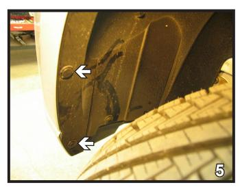
5. Remove two (2) push pins from the wheel well using a flat screwdriver. Do this to both sides of the vehicle. Set push pins aside to be reinstalled later.
