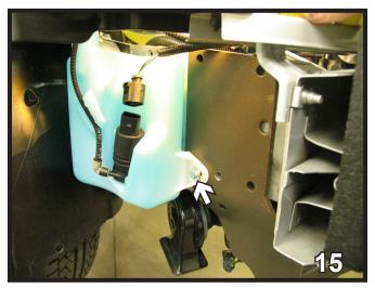
15. On the passenger side, do the same thing but there is an extra hole to reinstall the windshield washer tank in that hole use the longer 6MM bolt.
