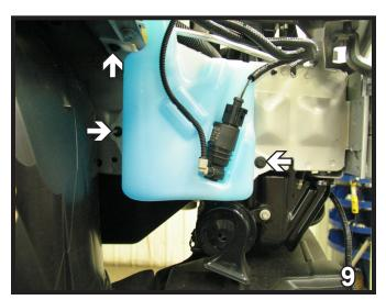
Using the 10MM socket, remove three (3) metric bolts from the windshield washer tank. Set bolts and tank aside to be reinstalled later.
