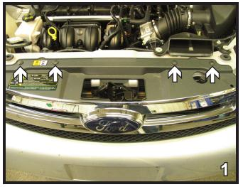
1. Remove four (4) Phillips push pins from radiator cover and lift to remove. Also remove grille assembly. Set push pins, radiator cover and grille aside to be reinstalled later.
