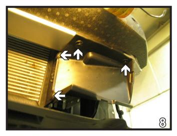
8. Using a flat screwdriver, remove four (4) push pins. Do this to both one sides of the vehicle. Remove the air dam. Set push pins and air dam aside to be reinstalled later.
