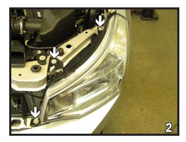
2. Using the 10MM socket, remove three (3) screws from the headlight assembly, disconnect electrical and pull forward to remove. Do this to both sides of the vehicle. Set screws and headlight assemblies aside to be reinstalled later.
