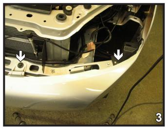
3. Remove two (2) push pins from upper corner of fascia. Do this to both sides of the vehicle. Set push pins aside to be reinstalled later.
