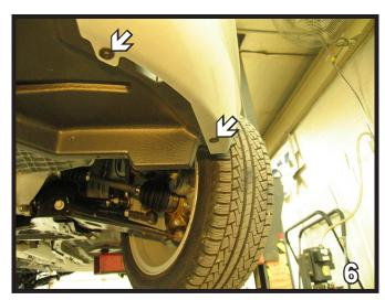
6. Using the 7MM socket, remove two (2) screws from the bottom corner of fascia. Do this to both sides of the vehicle. Set screws aside to be reinstalled later.
