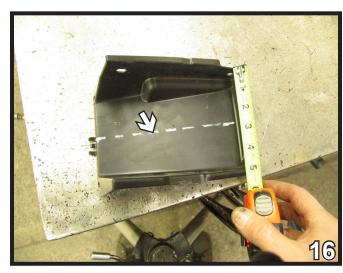
16. Trim the air dam, from the to edge take off 2-3/4". This allows clearance for the baseplate.
