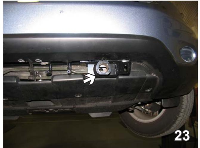
23. **2010 Model:** Trim the two outside bars completely off so that the baseplate tabs can come through. Do this on both sides.
