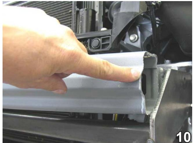
10. Using the reciprocating saw, cut the metal bumper to make it flush with the side of the frame rail, approximately 1/4" from the end of metal bumper. Do this to both sides of the vehicle. This clears the area for baseplate installation.
