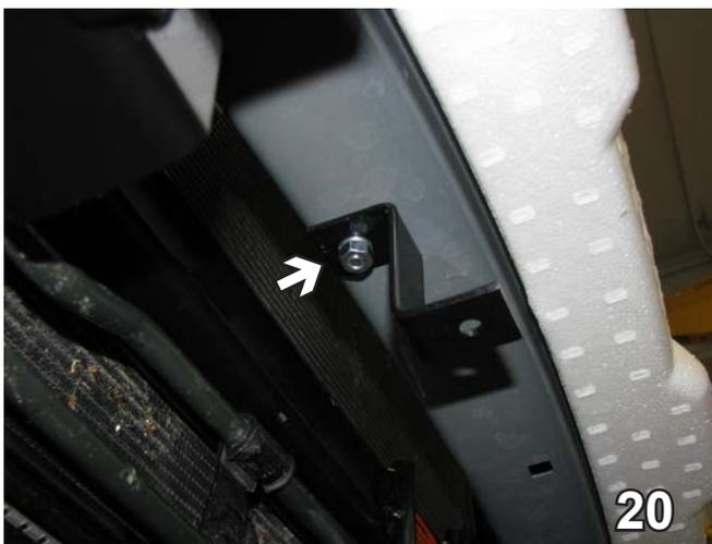
20. Attach the breakaway bracket to the underside of the metal bumper with a 1/4"-20 x 3/4" bolt and 1/4"-20 nut.
