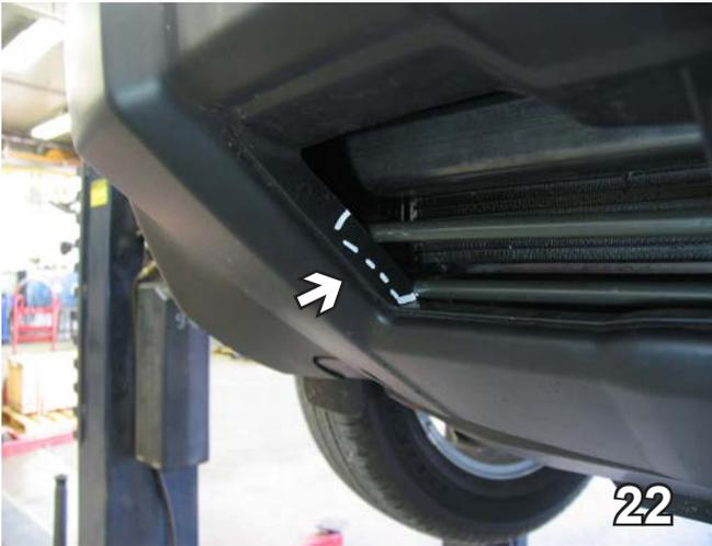
22. Align the fascia to its original position and, using the hack saw blade or utility knife, trim fascia contours to allow room for relocated coolant lines. Do this to both sides of the vehicle. Remove fascia.
