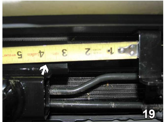
19. Measure 4" from the receiver tube to location position for the breakaway bracket. Drill a hole into the bottom of the metal bumper with 9/32" drill bit.
