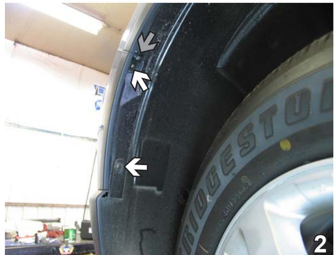
2. Just forward of front tire, inside the wheel well, remove two Phillips screws (see white arrows). Remove one pushpin on the corner of fascia, just above the upper Phillips screw (see grey arrow). Do this to both sides of the vehicle. Set screws and pushpins aside to be reinstalled later.
