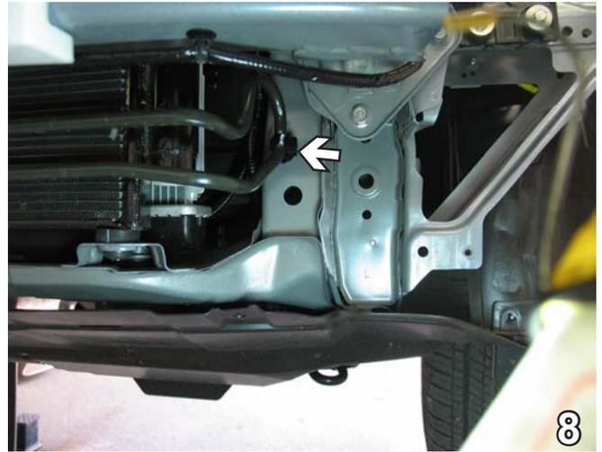
8. On driver's side, remove the coolant line clip from the front of lower frame support just below metal bumper. Do not remove clip from coolant line. Pull the driver's side end of coolant line over to the passenger side of vehicle to clear area for baseplate installation.
