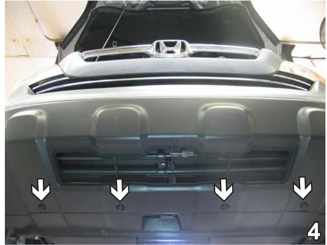
4. Remove four pushpins from the bottom of fascia. Pull fascia corners to the side, then forward to remove. Set pushpins and fascia aside carefully to be reinstalled later.
