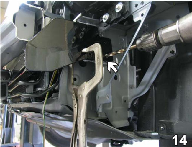
14. On side of frame rail, align baseplate to bottom of the flattened webbing and clamp in place with the vise grips. Using the baseplate as a template, drill four holes into the frame rail with the 13/32" drill bit. Insert two 3/8" nut plates through opening in frame rail end and align to top two holes. Install two 3/8-16 x 1 1/4" hex bolts and 3/8" lock washers to nut plates. Do not tighten. Install bumper. Now, tighten hex bolts. Do this to both sides of the vehicle.
