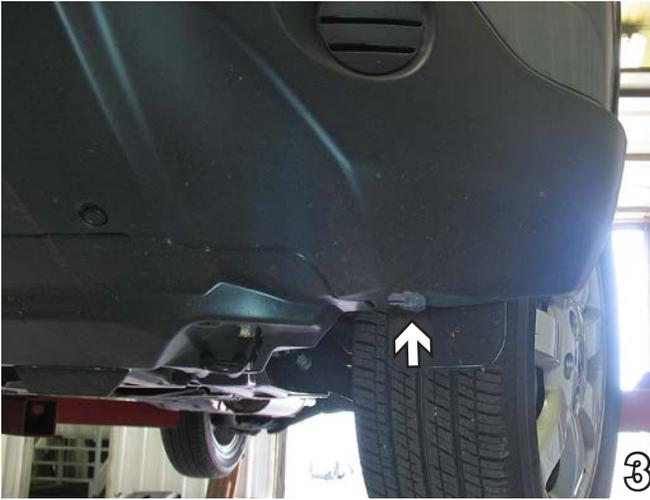
3. On driver's side, remove one metric bolt from the lower edge of fascia, just forward of front tire, using the 10mm socket. Do this to both sides of vehicle. Set bolts aside to be reinstalled later.
