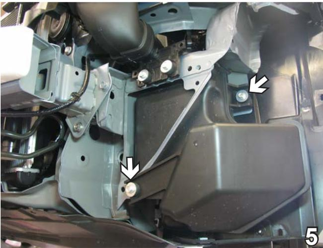
5. On the driver's side, remove two metric bolts from the air baffle using the 10mm socket. Pull air baffle down and out to the side of vehicle to remove. Set bolts and air baffle aside to be reinstalled later.
