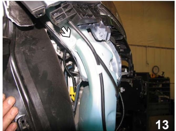
13. **2010 Model:** Remove one metric bolt from the back side of washer reservoir using the 10mm socket. Pull reservoir down and to the side to remove. Set bolts and reservoir aside to be reinstalled later.
