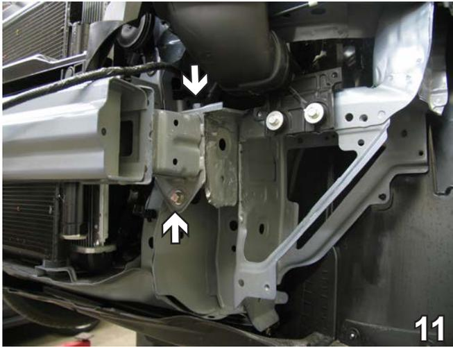
11. Using the 12mm socket, remove two metric bolts (one from the top and one from the bottom) of the metal bumper support. Do this to both sides of the vehicle. Remove the pins attaching the temperature sensor to the bottom of the bumper. Pull bumper forward to remove. Set bolts, bumper, pins and sensor aside to be reinstalled later.
