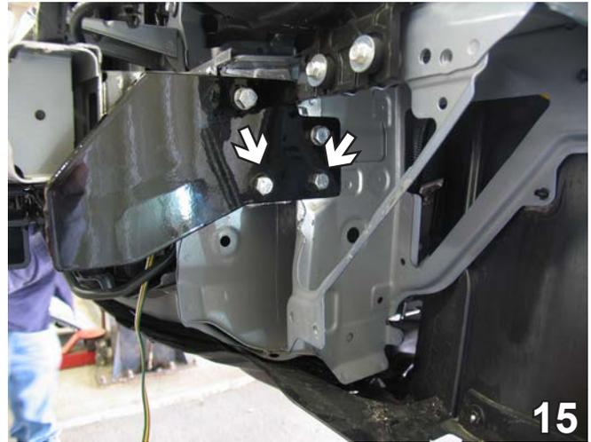
15. In lower drilled holes of baseplate, install two 3/8-16 x 1" hex bolts, 3/8" lock washers and 3/8-16 hex nuts and tighten. Do this to both sides of the vehicle.
