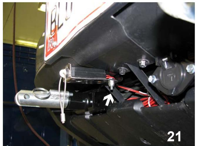
21. Attach the breakaway (not supplied) to the bracket with 1/4"-20 x 3/4" bolt and 1/4"-20 nut.
