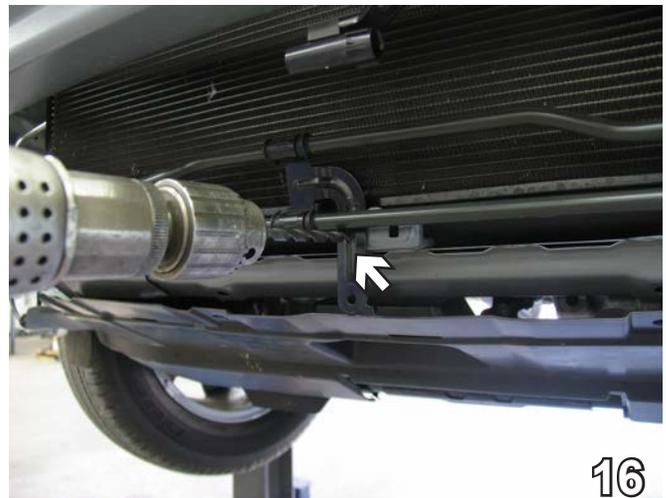
16. Relocate coolant line lower. Move bottom coolant line to just above original bolt hole for the bracket. Drill into the bracket using the 9/32" drill bit. Insert 10mm metric bolt into drilled hole and tighten.
