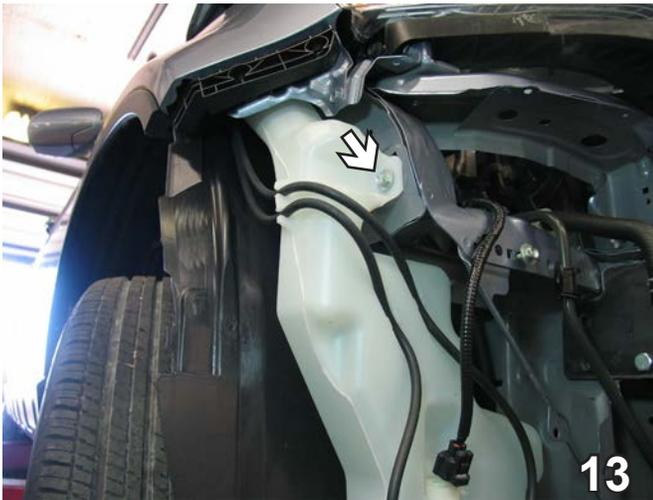
13. **2007-09 Models:** Remove one metric bolt from the side of washer reservoir using the 10mm socket. Pull reservoir down and to the side to remove. Set bolts and reservoir aside to be reinstalled later.
