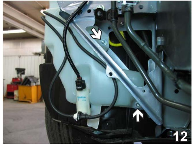
12. On the passenger's side, disconnect and plug the washer reservoir. Remove two metric bolts from the front of reservoir using the 10mm socket. Set bolts aside to be reinstalled later.
