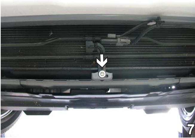
7. Using the 10mm socket, remove one metric bolt from the coolant line bracket at the bottom of radiator. Set bolt aside to be reinstalled later.
