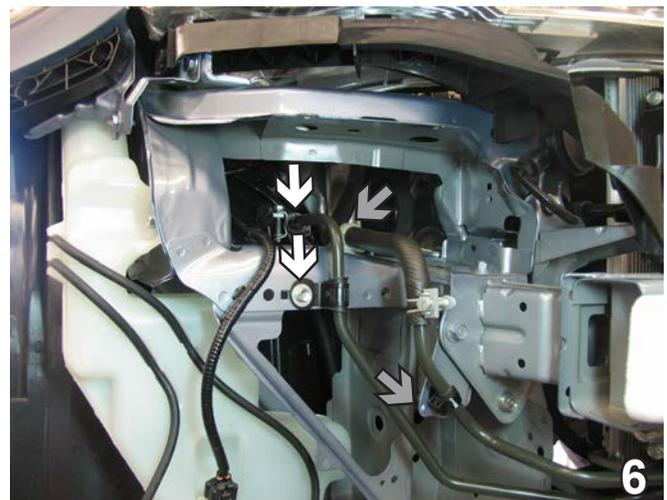
6. On passenger's side, on coolant line closest to washer reservoir, remove one metric bolt using the 10mm socket (see lower white arrow) and disconnect one clip from line (see upper white arrow). On the coolant line closest to frame, disconnect two clips (see grey arrows). The two upper clips will remain on vehicle and the two lower clips are to remain on coolant lines.
