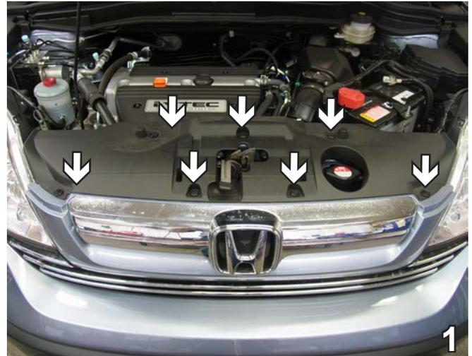
1. Remove seven pushpins from the top of the radiator cover. Pull radiator cover forward to remove. Set radiator cover and pushpins aside to be reinstalled later.
