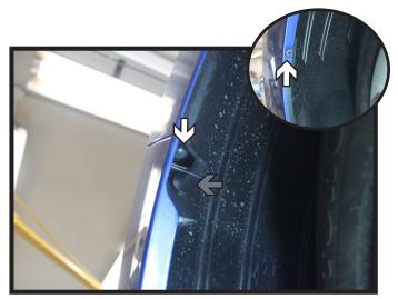
3. In the wheel well, remove the push pin just below the fascia joint (gray). Using a Phillips screwdriver, remove the two (2) screws (white). There is one (1) at the fascia joint and one (1) along the outer edge below the joint. Do this on both sides of the vehicle.
