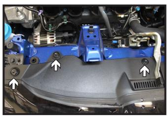
On the passenger side, remove the three
