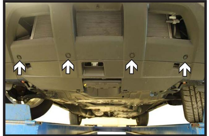
5. Remove the four (4) push pins that are located under the fascia.
