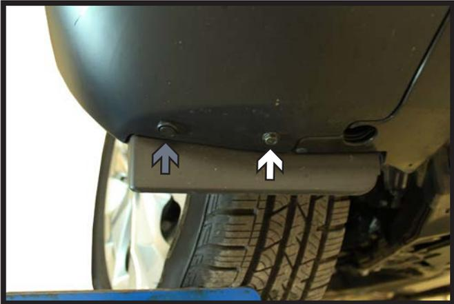
4. Remove the one (1) screw (white) and one (1) push pin (gray) that are on the under side of the fascia, in front of the tire. Do this on both sides of the vehicle.
