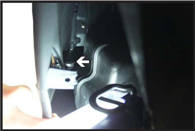
3. Behind the wheel well liner, remove the push pin that is located along the lower outside edge. Do this on both sides of the vehicle.
