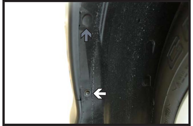
2. Using a Phillips screwdriver, remove the screw at the bottom of the wheel well (white). Then remove the two (2) push pins located above the screw (gray). Do this on both sides of the vehicle.
