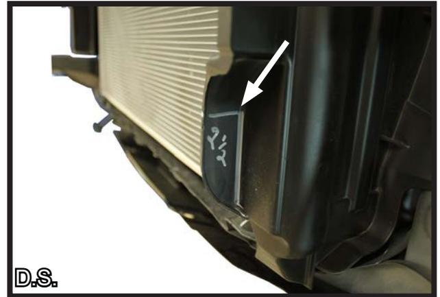
12. On the passenger side, cut straight down to remove the bottom portion. On the driver side, notch up 2-1/2" and straight out.
