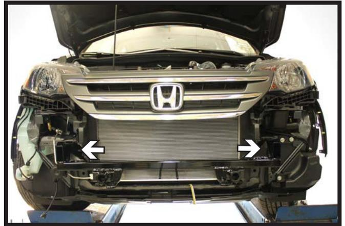
16. Slide the baseplate tubes into the rectangular tubing of the vehicle frame.
