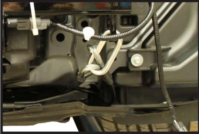
23. Attach the permanent baseplate safety cables to the provided convenience link on the baseplate. The photo shows the recommended installation of the cables to frame of vehicle. Additional options may interfere with suggested mounting; in this case, secure the cables to a solid piece of the frame as described in the instructions included with the permanent baseplate safety cables. Be sure the safety cables do not rub against any hoses or moving parts. Do this on **BOTH** sides of the vehicle.
