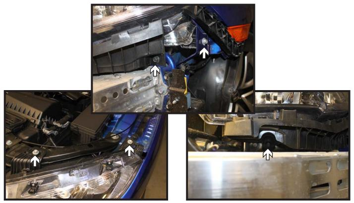
7. Using a 10MM socket, remove the five (5) screws from the headlight. Disconnect all electrical lines and set aside. Do this on both sides of the vehicle.
