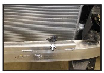
6. Remove the temperature sensor from the bumper and set aside.
