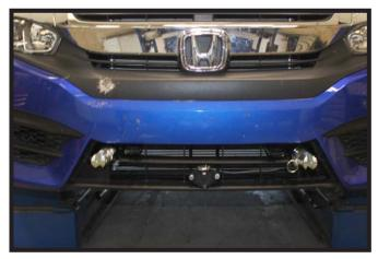
14. Hold the fascia as close to its original position, mark and trim the fascia around the convenience links and attachment tabs. Reinstall the headlights, fascia and fascia cover.
