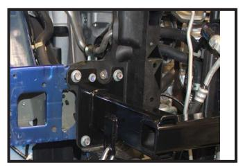
11. Install the baseplate to the vehicle using the existing hardware. Fully tighten all fasteners.
