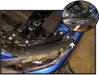
2. Remove the push pin from the corner of the chrome strip and unsnap from the vehicle. Do this on both sides of the vehicle.
