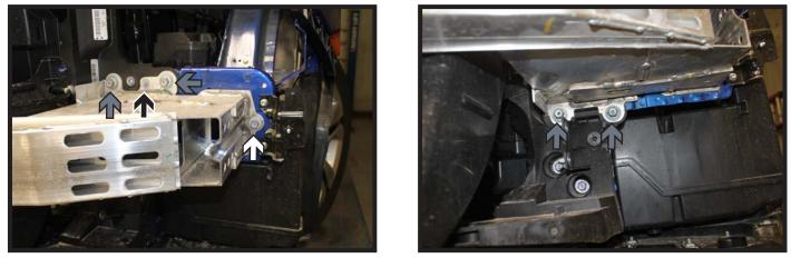
8. Using a 14MM socket, remove the four (4) bolts from the bumper (gray). There are two (2) each on the top side and underside. Using a 12MM socket, remove the bolt from the side of the bumper (white). Using a 10MM socket, remove the bolt from the top side of the bumper (black). Do this on both sides of the vehicle. Set the bumper aside it will not be reinstalled.
