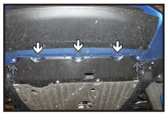
Using a 10MM socket, remove the screw (gray) from the underside of the fascia. Then remove the two (2) push pins (left photo). Do this on both sides of the vehicle. Using a T30 Torx, remove the two (2) screws towards the center (gray). Then remove the three (3) push pins (right photo).
