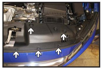
1. Remove the ten (10) push pins from the fascia cover. There are five (5) on each side. Set the cover aside.
