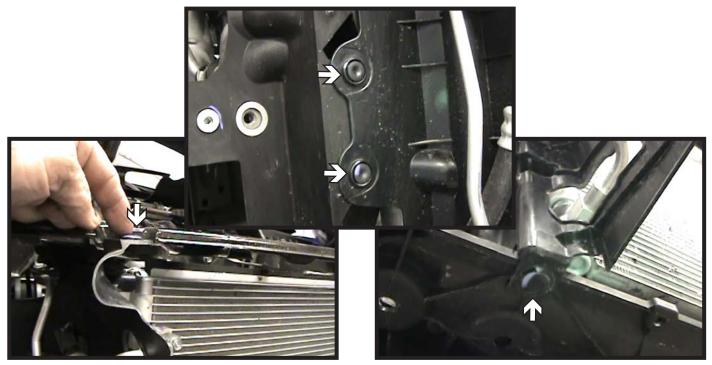
9. Remove the plastic shielding from the vehicle by removing the four (4) push pins. There is one (1) on top, two (2) along the side and one (1) at the bottom. Do this on both sides of the vehicle. The shielding will not be reinstalled.
