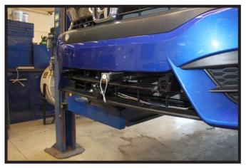
15. **Optional Breakaway:** In the desired location, drill a 1/4" hole thru the fascia lip. Install the breakaway to the fascia with the 1/4" hardware provided.
