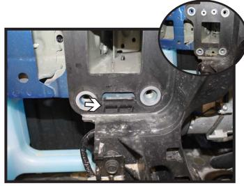
10. Using a reciprocating saw, trim the hook at the lower bumper bolt location flush with the frame. Do this on both sides of the vehicle.
