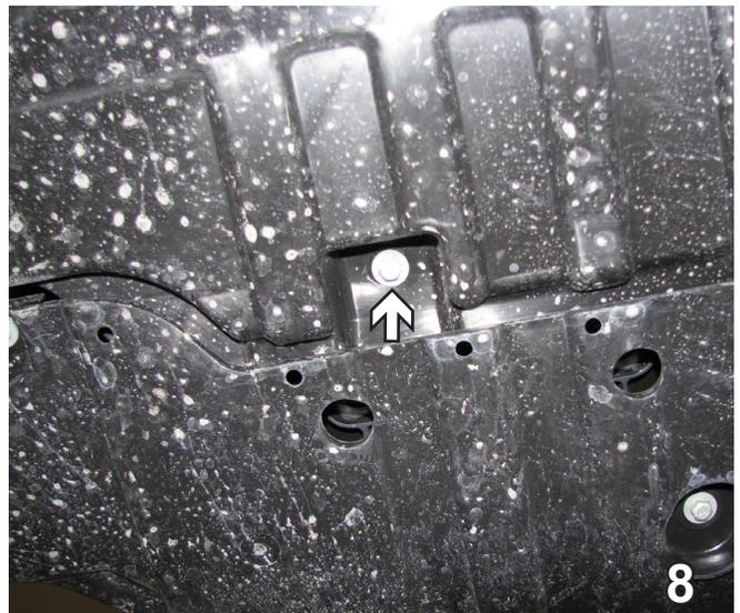
8. Using a 10MM socket, remove three (3) bolts underneath across the front of the back plastic cover. One bolt on each side and one in the middle. Set bolts and plastic aside to be reinstalled later.
