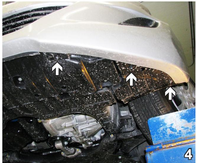
4. Using a Phillips screwdriver, remove three (3) plastic Phillips push pins from just forward of the front tire along the bottom edge of fascia. The fascia is then ready to be removed from the vehicle by pulling fascia ends out to the side to release and then pulling it forward. Do this to both sides of the vehicle. Set fascia and push pins aside to be reinstalled later.
