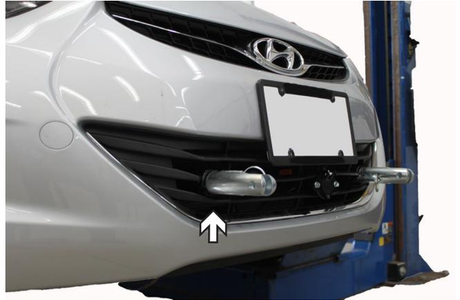
31. Reinstall the bumper and plastic cover. Trim the fascia as needed to clear the baseplate attachment tabs then reinstall. Reconnect the cables and the electrical plugs.
