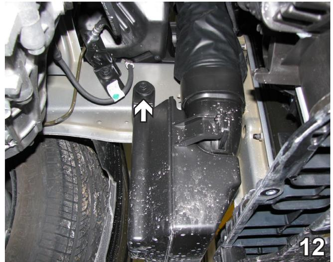
12. On the driver side underneath the vehicle, using a 10MM socket remove the bolt. Set the air baffle and the bolt aside to be reinstalled later.
