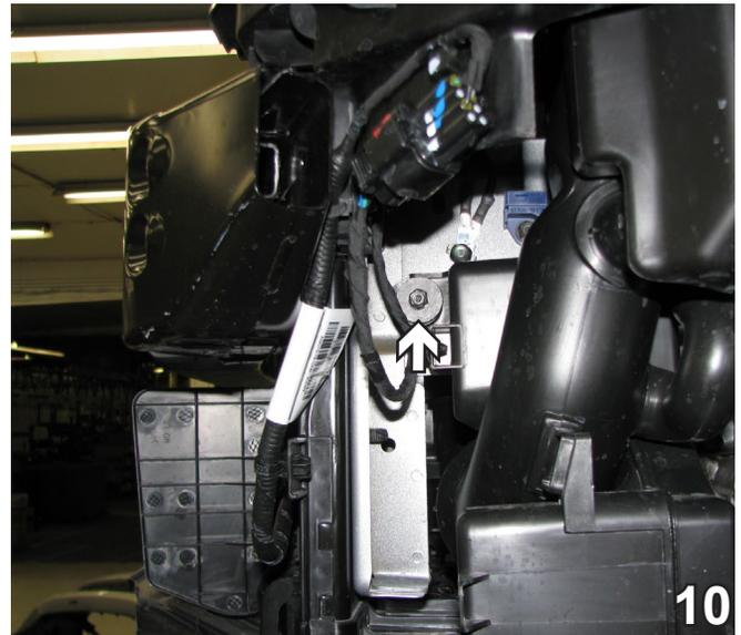
10. On the driver side, using a 10MM socket remove one bolt on the outside of the air baffle.
