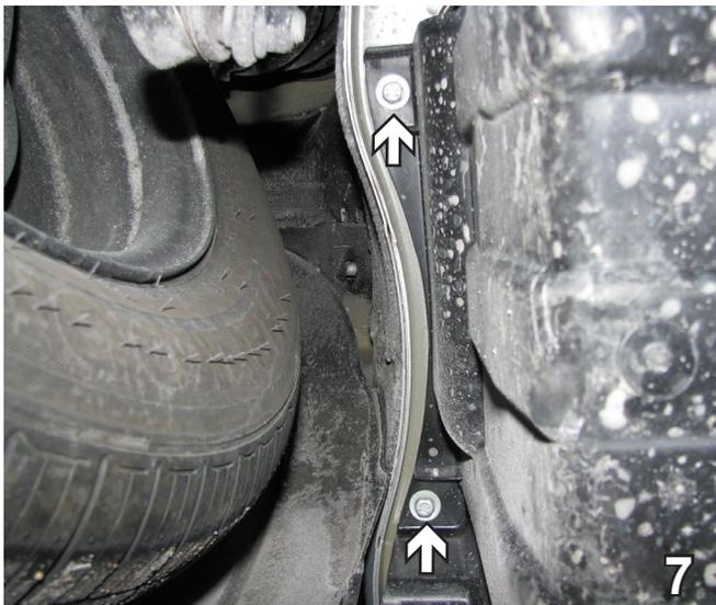
7. Using a 10MM socket, remove two (2) bolts underneath on the side of the back plastic cover. Do this on both sides of the vehicle. Set bolts aside to be reinstalled later.
