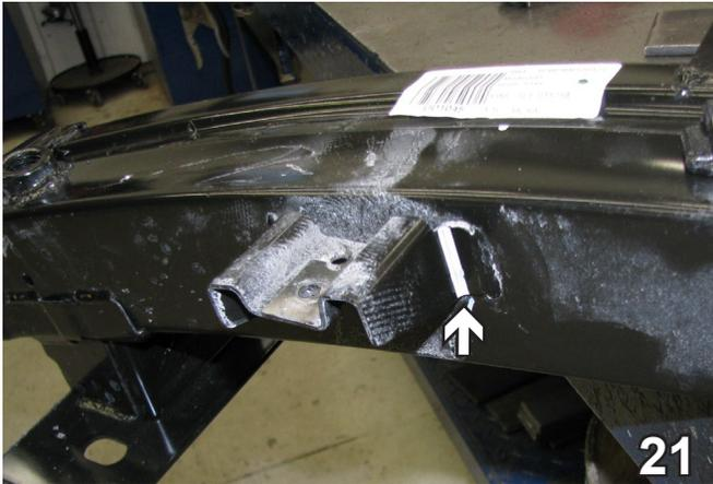
21. Cut the horn bracket off of the bumper on the passenger side. It will be reinstalled in a different location.
