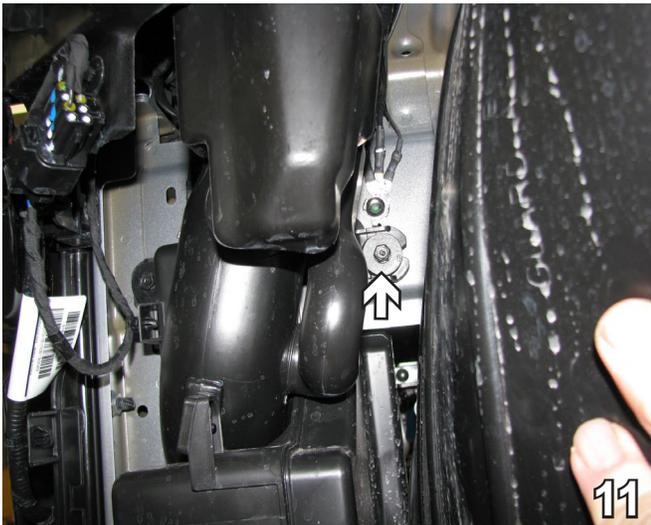
11. On the driver side, using a 10MM socket, remove the bolt from the back side of the air baffle. Set the bolt aside to be reinstalled later.
