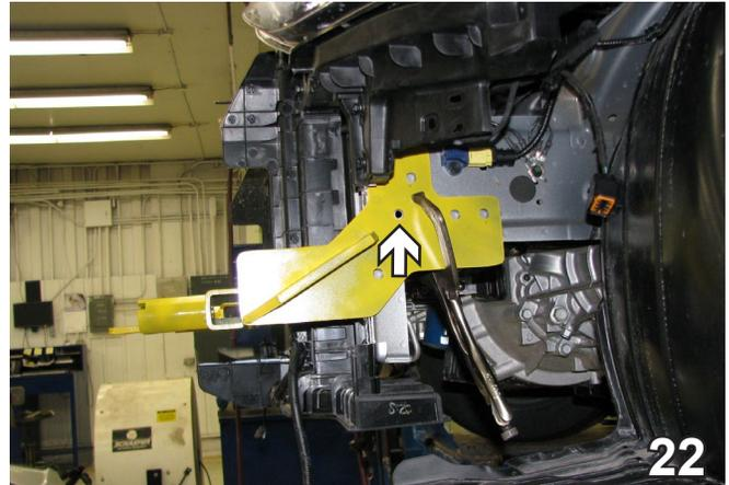
22. Slide the baseplate up so it aligns with the existing hole on the driver's side. Clamp into place with the large vise grips.
