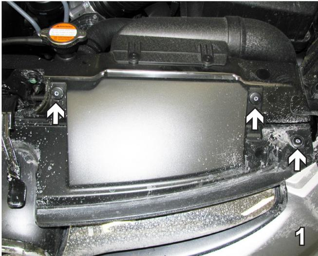
1. On the driver side using a Phillips screwdriver, remove three (3) push pins from the top of the fascia. Set pins aside to be reinstalled later.
