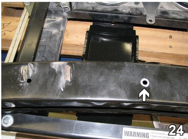
24. On the bottom of the bumper using a 13/32" drill bit, drill out the existing hole on the passenger side all the way through. This hole will be used later on for the breakaway bracket installation.
