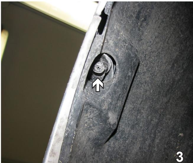
3. Using a 10MM socket, remove the metric bolt from in front of the tire. Do this to both sides of the vehicle. Set bolts aside to be reinstalled later.
