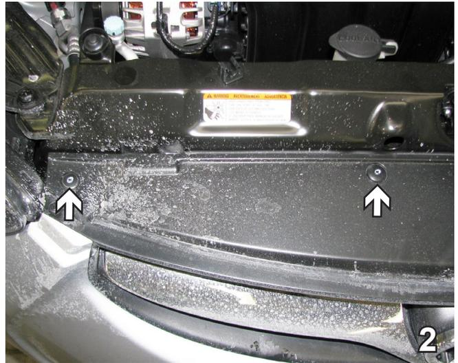
2. On the passenger side using a Phillips screwdriver, remove two (2) push pins from the top of the fascia. Set pins aside to be reinstalled later.
