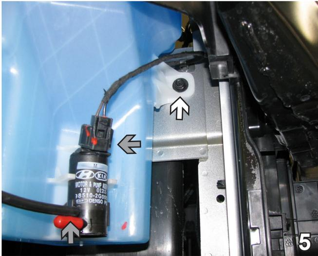
5. On the passenger side, unplug the hoses from the windshield washer reservoir and cap (gray arrows). Using a 10MM socket, remove the bolt on the side (white arrow). Set the bolt aside to be reinstalled later.
