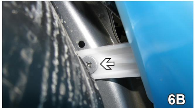
6. Using a 10MM socket, remove the metric bolt in the back (6A). Using a Phillips screwdriver loosen the screw on the top (6B). Set washer reservoir and bolts aside to be reinstalled later.
