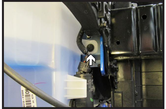
9. Using a 10MM socket, remove the two (2) bolts securing the windshield wiper fluid reservoir. Disconnect and plug all lines, and set the reservoir aside.
