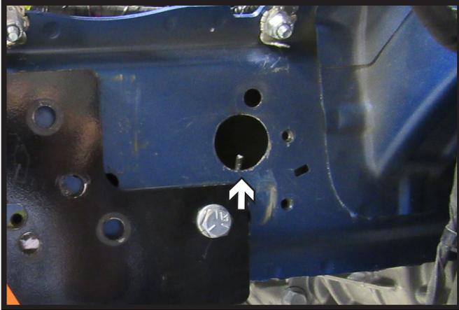
13. On each side of the frame right above the baseplate drill an 1-1/4" hole using a hole saw to use as the access hole for the nut plates with 14" wire.
