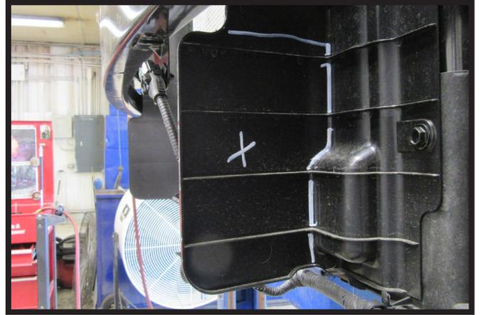
12. Using a reciprocating saw, trim the marked areas on both sides of the plastic shielding on the bumper.
