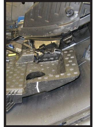
18. Using a reciprocating saw, trim the marked areas on both sides of the fascia.
