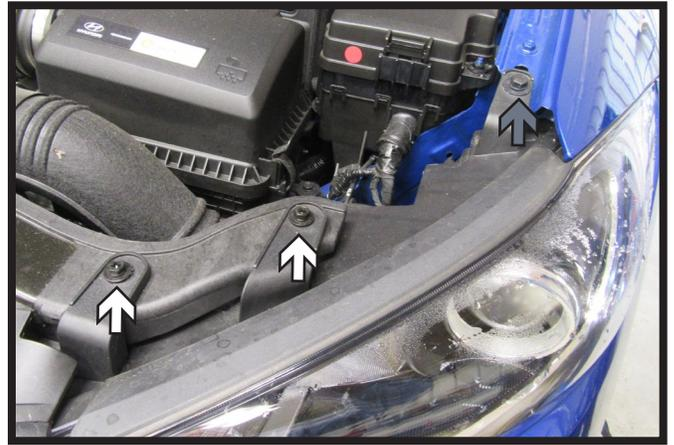
2. Using a 10MM socket, remove the two (2) bolts from above the headlights (white). Using a 12MM socket, remove the one (1) upper bolt (gray). Do this for both sides of the vehicle.
