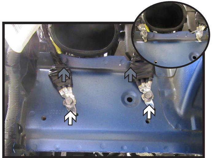
10. Using a 10MM socket, remove the two (2) bolts on the passenger's side bumper horn (white). Using a 1/4" drill bit, bore the upper existing hole out (gray). Bolt the connections in this hole, as pictured above.
