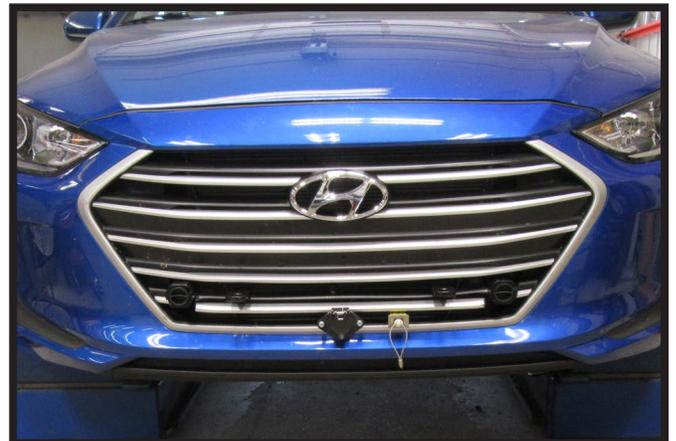
20. Hold the fascia as close to its original position, mark and trim the fascia around the convenience links and attachment tabs. Reinstall the windshield wiper fluid reservoir, horns, fascia and fascia cover.
