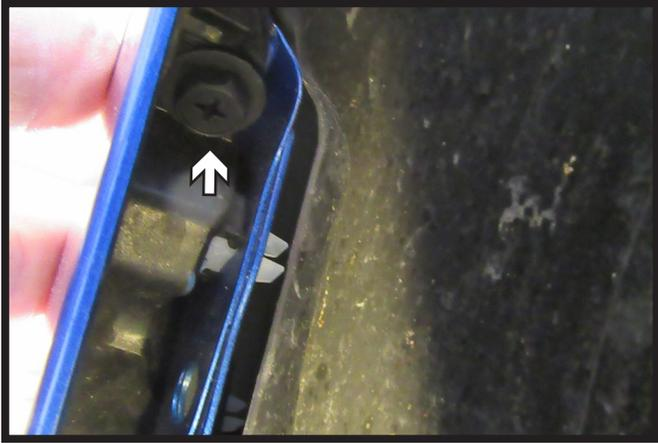
4. Using a 10MM socket, remove the one (1) bolt from the upper part of the wheel well. Do this for both sides of the vehicle.
