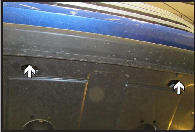
3. Underneath the vehicle, remove ten (10) push pins. There are two (2) towards the front, and four (4) on both sides.
