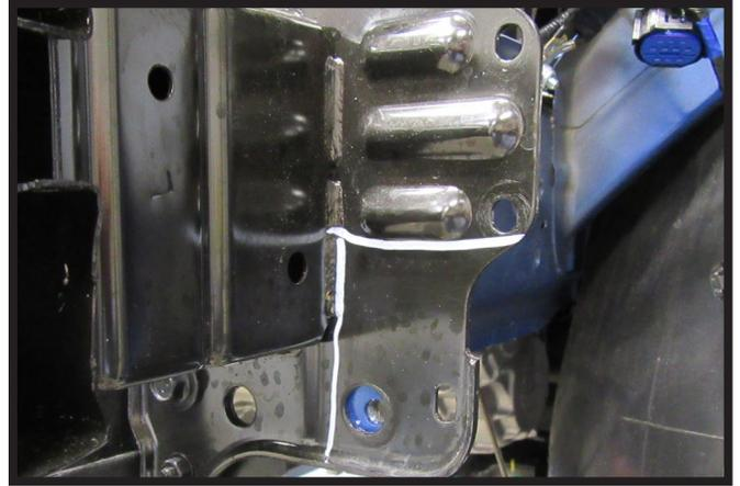
15. Using a reciprocating saw, trim the marked areas on both sides of the bumper horn.
