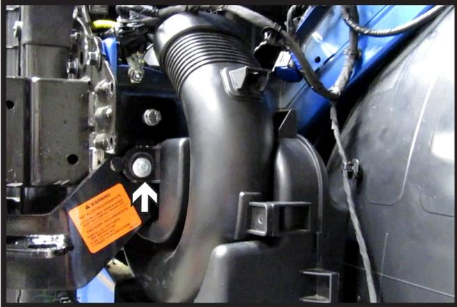
17. When reinstalling the air baffle, use the supplied 3/8" hardware to secure it through the baseplate hole.
