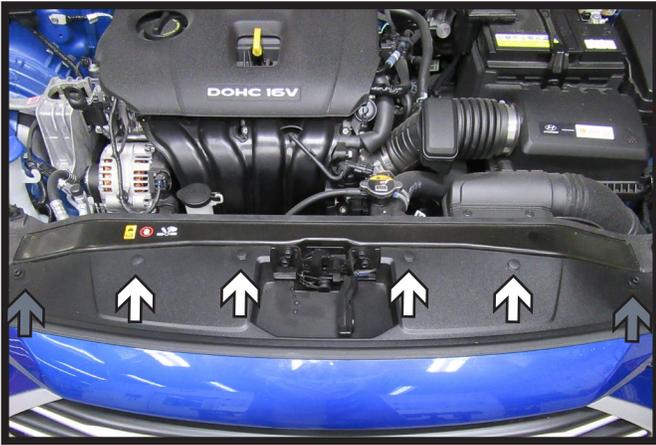
1. Remove the four (4) push pins from the top of the fascia cover (white). Using a 10MM socket, remove the two (2) bolts from the fascia cover (gray).
