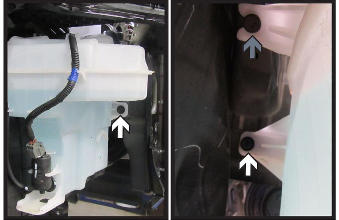
7. Using a 10MM socket, remove the two (2) bolts (white) and one (1) screw (gray) from the windshield washer fluid reservoir on the passenger side of the vehicle. Remove fluid lines and plug. Remove reservoir and set aside to be reinstalled later.
