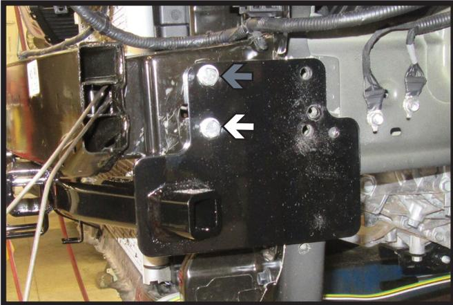
13. Start a 3/8" bolt with lock washer and nut plate in the bottom front hole (white). Using a 3/8" drill bit, drill the top front hole and install the 3/8" bolt with lock washer and nut plate (gray). Remove the 6MM bolt from the existing back hole. Do this on both sides of the vehicle.
