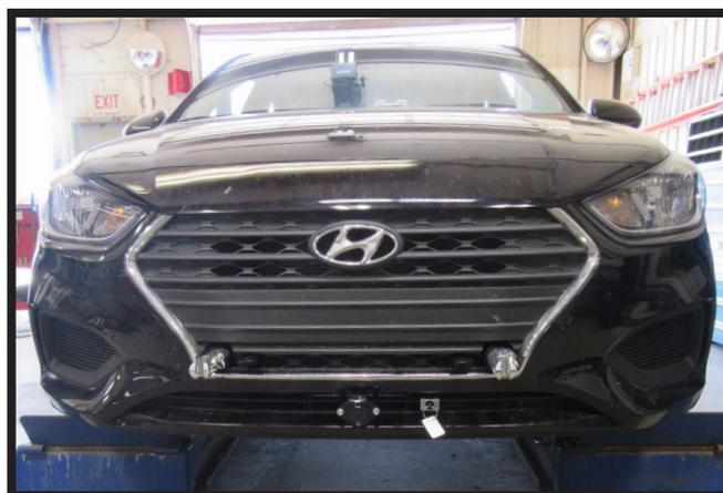
19. Reinstall the windshield washer fluid reservoir. Hold the fascia as close to its original position, mark and trim the fascia around the convenience links and attachment tabs. Reinstall the belly pan and fascia.
