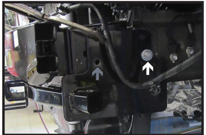
12. Slide the baseplate into place, start a 6MM bolt with hardware into the existing back hole (white). Clamp baseplate into place using a large vise grip. Using a 3/8" drill bit, drill out the front bottom hole (gray). Do this on both sides of the vehicle.
