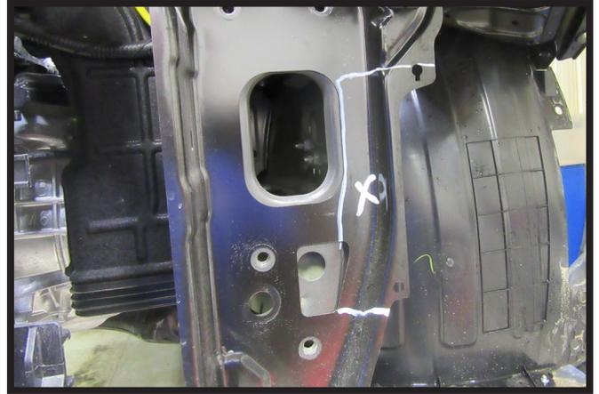
10. Using a reciprocating saw, remove the indicated areas on each side of the vehicle so that it is flush with the frame.
