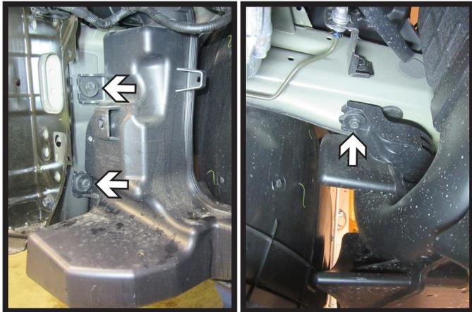
8. Using a 10MM socket, remove the three (3) bolts from the air intake on the driver side of the vehicle. Remove the air intake and set aside to be reinstalled later.
