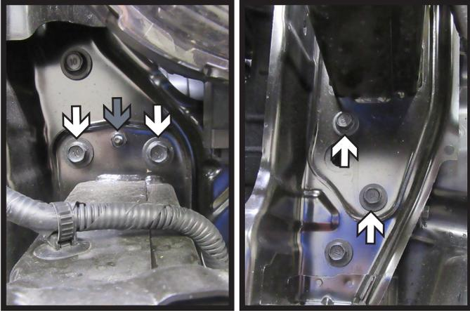
6. Using a 12MM socket, remove the four (4) bolts (white) from the bumper. Using a 10MM socket, remove the one (1) bolt (gray) on the top of the bumper. Do this on both sides of the vehicle. Unclip the wire loom from the bumper. Remove bumper and set aside to be reinstalled later.
