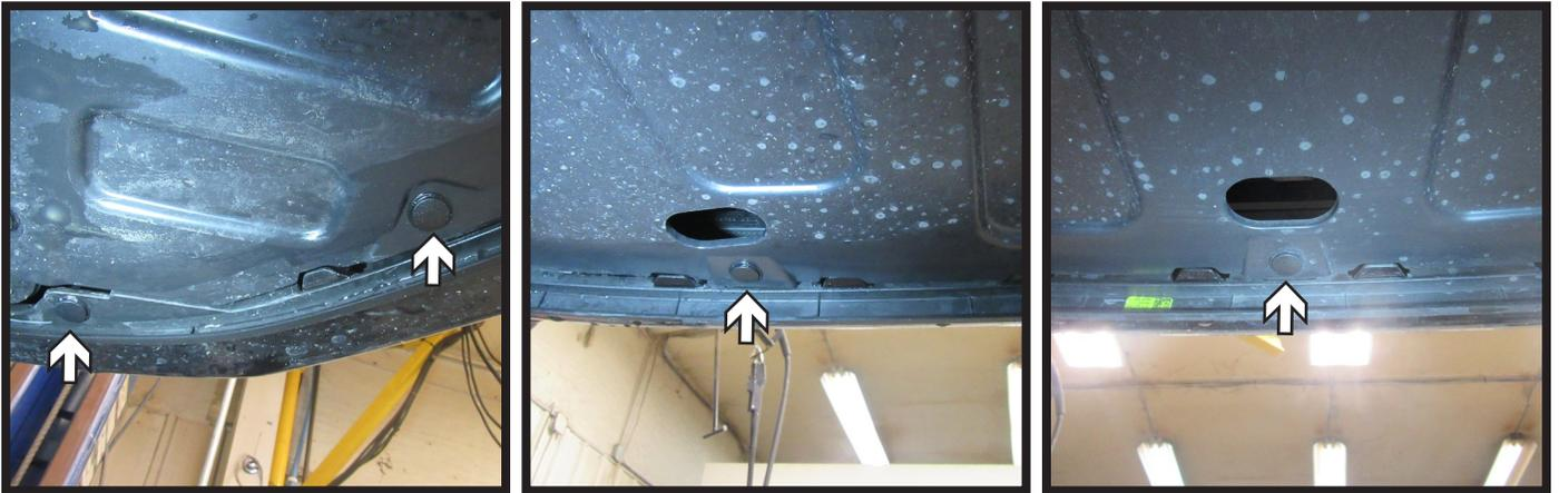
4. Remove the seven (7) push pins from the underside of the fascia. There are three (3) push pins on each side of the vehicle and one (1) in the center.
