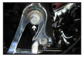
4. **Trucks with Tow Hooks:** Using an 18MM socket remove the front bolt (white), [to be reinstalled after tow hook is removed] and then using a 21MM socket remove the back bolt (gray) attaching the tow hook to the frame. Do this on both sides of the vehicle. The tow hooks will not be reinstalled.
