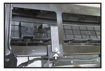
11. Optional: Remove the existing bolt from either side of the vehicle and install the breakaway bracket. Cut a hole in the fascia to allow room for the breakaway switch.
