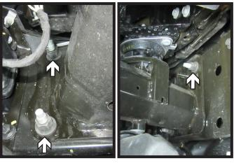
2. Using an 18MM socket, remove the three (3) bolts from the bumper. Do this on both sides of the vehicle.
