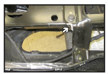
10. Using a reciprocating saw, remove the indicated area on the back side of the fascia to allow room for the baseplate. Do this on both sides of the vehicle.
