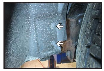
Using an 8MM socket loosen the two
