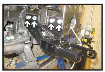
7. Using a 1/2" drill bit, drill the four (4) holes on the side of the frame starting with the back hole. Install 1/2" bolts with lock washers and whiz nuts. Do this on both sides of the vehicle.
