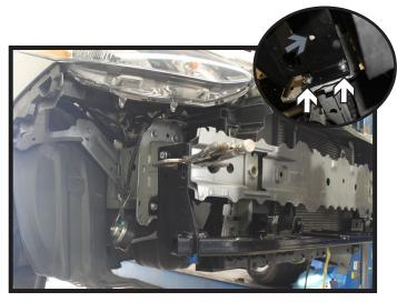
9. Position the baseplate onto the vehicle, start the four (4) 8MM bolts with 5/16" lock and flat washers into the existing frame extension holes (white). There are (2) on each side.
