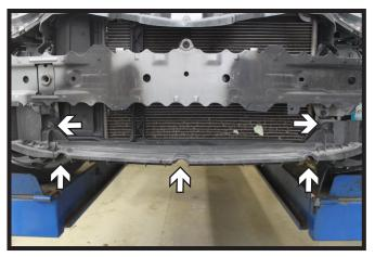
6. Using a 10MM socket, remove the five (5) screws from the lower shrouding. The shrouding will not be reinstalled.
