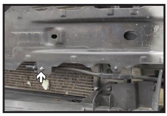
5. Remove the temperature sensor from the bumper and move it aside.
