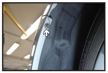
Using a 8MM socket, remove the screw from the edge of the wheel well. Do this on both sides of the vehicle.
