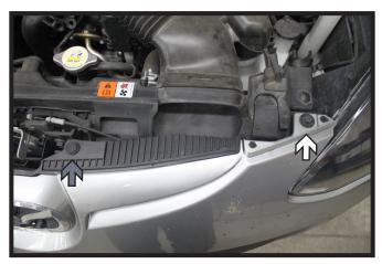
Using a 10MM socket, remove the screw from the top edge of the fascia (white).
