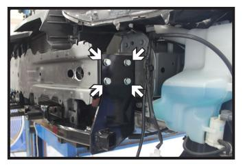
10. Using a 13/32" drill bit, dril the eight (8) holes on the sides of the baseplate thru the frame. There are four (4) on each side. Install 3/8"-16 x 1-1/4" bolts with 3/8" lock washers into the holes and secure with 3/8" nut plates on the inside of the frame.
