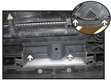
3. Using a 8MM socket, remove the six (6) screws from the Underside of the fascia. There are two (2) on each side (inset) and two (2) in the middle. Pry the corners of the fascia away from the vehicle. Disconnect all electrical connections and pull the fascia off from the vehicle.
