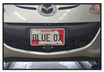
12. Hold the fascia as close to its original position, mark and trim the fascia around the convenience links and attachment tabs. Reinstall the fascia.
