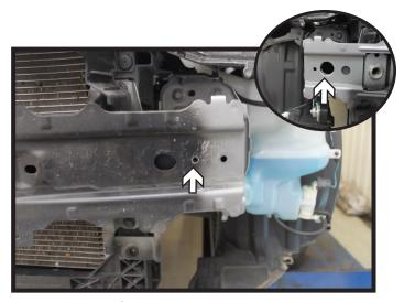
7. Using a 1/4" drill bit, drill a pilot hole as shown in the bumper. Using a 1-1/4" hole saw, drill out the pilot hole thru the bumper and frame for nut plate access. Do this on both sides of the vehicle.
