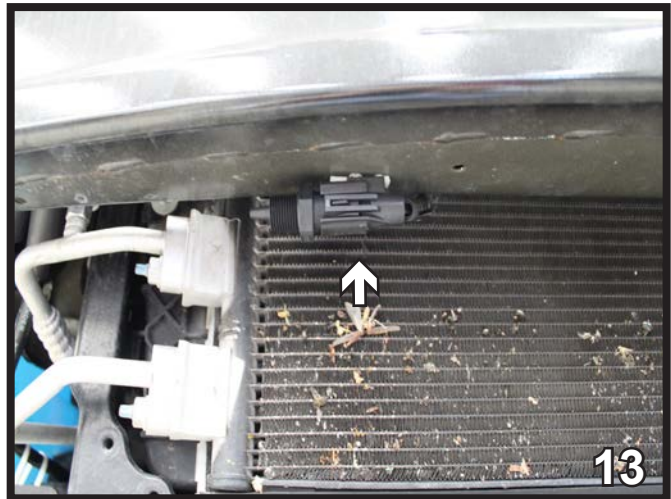
13. After bumper is reinstalled, when applicable, relocate temperature sensor on passenger's side to the bottom of the bumper using existing holes.
