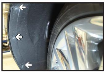
Using a 5.5MM socket, remove the three (3) screws just forward of the front tire in the wheel well. Do this to both sides of the vehicle.
