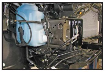
Reinstall the washer fluid reservoir, cruise control box. Hold the fascia as close to its original position. Mark and trim for the attachment tabs and conveinence links. Reinstall the fascia.
