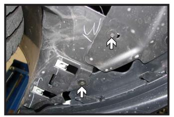
3. Using a 5.5MM socket, remove the two (2) screws from underneath the front edge of fascia. Do this to both sides of the vehicle.
