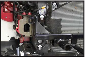
14. Reinstall the existing bolts to the top and bottom of the radiator support. Do this on both sides of the vehicle.
