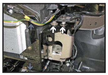
Place baseplate on top of frame and line up the holes in the baseplate with the two (2) existing holes on top of the frame. Reinstall the four (4) existing bolts from step 6, two (2) on the top (white) and (2) on the face (gray). Do this to both sides of the vehicle.
