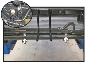
15. Remove coolant line brackets from the back side and relocate to the front of the coolant line. Using the bracket as a template, drill 1/4" holes into the lower cross member and install 1/4"-20 x 3/4" bolts and 1/4"-20 nuts on the back side of the cross member (white). Reinstall the bolt located on the side of the
