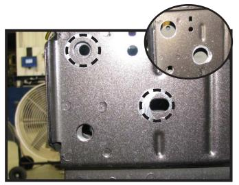
Using a 1 1/4" hole saw, drill two (2) 1-1/4" holes into the frame, utilizing the two (2) existing holes in the side of the frame. This gives an access hole to tighten fasteners. Do this to both sides of the vehicle.
