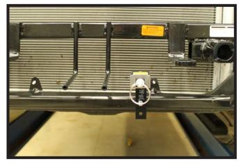
17. OPTIONAL: Install the breakaway bracket and breakaway on the driver's side of the vehicle between the convienence link and electrical rods. Drill a 1/4" hole into the frame located below the radiator. Attach the bracket to frame of vehicle with 1/4"-20 x 3/4" bolt and 1/4"-20 nylon nut. Attach the breakaway to the bracket with a 1/4"-20 x 3/4" bolt and 1/4"-20 locking nut.
