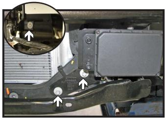
5. If vehicle is equipped with ACC, on the drivers side only, using an 8mm socket remove the two (2) bolts from the front and the one (1) on the back side of the cruise control box.
