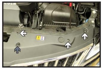
1. Remove the three (3) push pins (white) and then, using a 10MM socket, remove the one (1) screw (gray) from the plastic radiator cover. Do this to both sides of the vehicle.
