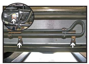
On the passenger side front of the vehicle, using a 10MM socket remove the two (2) bolts (white) from the lower coolant line. Then using a 8MM socket, remove the one (1) bolt (gray) located on the side of the vehicle. The lower coolant line now can be swung out of the way.
