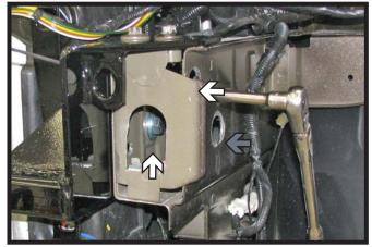
13. Align lower base plate holes to the existing holes. They may need to be reamed out using a 13/32" or 17/32" drill bit. Install a 3/8"-16 x 1" bolt, 3/8" lock washer, 3/8" flat washer and a 3/8" nut w/wire into the front holes and tighten down (white). Then install a 1/2"-13 x 1" bolt, 1/2" lock washer, 1/2" flat washer and a 1/2" nut plate into rear hole (gray). Do this to both sides of the vehicle.
