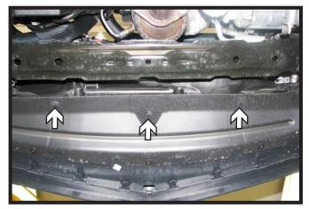
4. Remove the three (3) push pins that are located in the center of vehicle on the underside of the fascia. Then on the corners of the fascia pull out to the side and forward to remove. Set fascia aside.
