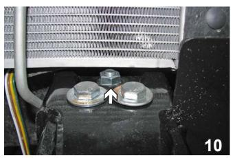
Insert 1/2-13 x 2 1/2" hex bolt into the back hole bottom side up with three 1/2" flat washers on the bottom and attaches with a 1/2-13 whiz nut on the top side. Do this on both sides. Tighten with Loctite Red.
