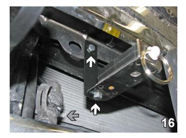
16. **Optional:** Install the breakaway bracket in the existing hole on the passenger side next to the license plate. Insert a 1/4-20 x 3/4" hex bolt with 1/4-20 hex nut. Also attach the breakaway to the bracket with a 1/4-20 x 3/4" hex bolt with 1/4-20 hex nut.
