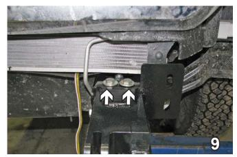
Slide the baseplate over the frame rail, tabs to the inside. Align with the top holes. Insert 1/2-13 x 3 1/2" hex bolts with 1/2" flat washers on the top and bottom and 1/2-13 hex nuts in the front holes. Do this on both sides. Tighten with Loctite Red.
