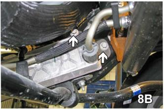
Using a 13MM socket remove the three metric bolts from the coolant transfer box on the passenger side to be reinstalled later. Pull the box out of the way so that the side holes can be drilled in step 12 using the baseplate as a template.
