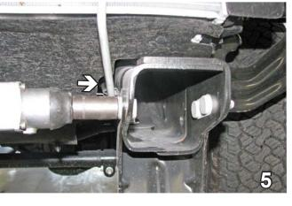
5. On the driver's side, it will be necessary to pull the Christmas tree pin from the coolant line bracket that goes into the frame in order to position the baseplate. It will be reinstalled later.
