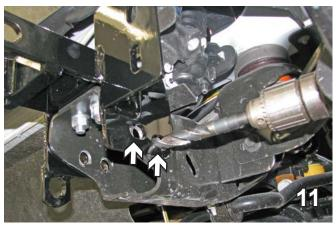
11. With the baseplate as a template, use a 5/8" drill bit to ream out the holes on both sides of the frame rail if needed. Do this on both sides of the vehicle.
