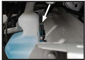
17. Place seven (7) 1/4" flat washers behind the reservoir on the inner most side prior to tightening the existing bolts.
