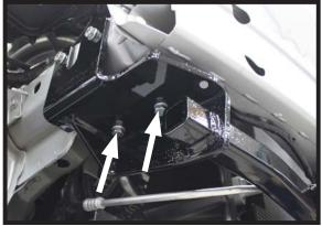
11. Using a 13/32" drill bit and the baseplate as a template, drill the bottom, back two (2) holes.
