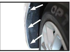
Using a 5.5MM socket, remove the three (3) bolts in the wheel well area. Do this on both sides.
