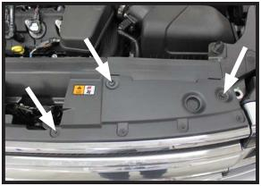
Using a 10MM socket, remove the two (2) bolts and push pins that are located in the front area, one (1) per side. There are eight (8) bolts along the front that also need to be removed using a 5.5MM socket.
