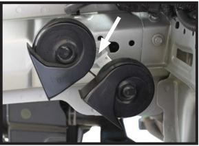
8. On the driver's side, remove the horn using an 8MM socket.
