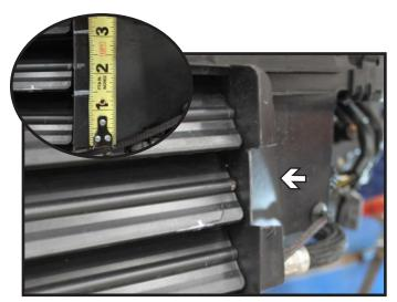
10. Hold up the baseplate to the vehicle and mark the shutter for cutting. The dimensions should be roughly 1-1/2" from the bottom and 3-1/4" to top of the cut. Trim both ends of the shutter to clear the baseplate.
