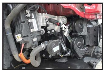
5. **Energi Only:** On the passenger side, using a 10MM socket, remove the screw from the bracket for baseplate installation clearance.
