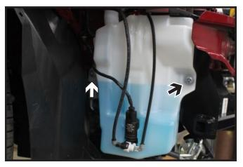
15. On the passenger side, reinstall the washer fluid reservoir. Reuse one (1) of the existing screws on left side (white). Then a 3/8"-16 x 1" bolt, 3/8" flat washer and 3/8" lock nut on the right side (black).
