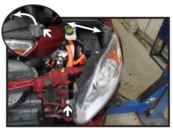
Using a T27 Torx, remove the two (2) screws from the front and back of the headlight. Lift up on the rear of headlight to release and unhook the wiring. Set the headlight aside. Do this on both sides of the vehicle.
