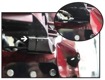
14. On the passenger side, trim the plastic flange above the baseplate for clearance of the washer fluid reservoir.
