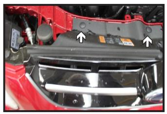
Remove the two (2) push pins from the top back edge of the fascia. Do this on both sides of vehicle.
