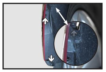
Using a T27 Torx, remove the two (2) screws from the outer edge of the wheel well (white). Above the screws where the fascia meets the fender remove the push pin (gray). Do this on both sides of the vehicle.
