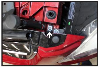
Using a T27 Torx, remove the inner screw behind the headlight from the fascia. Do this on both sides of the vehicle.
