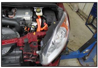
Plug in and reinstall the headlights on both the driver and passenger sides. Secure any loose wiring.
