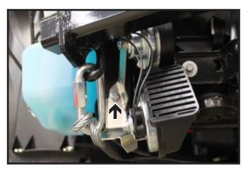
17. On the passenger side, reinstall the horn to the vehicle. Use one of the existing holes on the frame below the baseplate with a 1/4"-20 x 3/4" bolt and 1/4" nylon nut. Bend the bracket if needed to insure that the horn drains if exposed to water.
