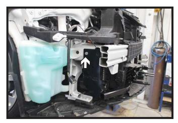
11. Using the existing holes in the frame, pin the rear baseplate holes to the frame with 3/8"-16 x 1-1/4" bolts and 3/8" lock washers.
