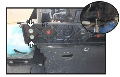
10. Using a 13MM socket, remove the two (2) screws from the support (white). Move the support inwards and ream out the existing hole (gray) with a 1/2" drill bit (inset).
