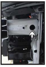
9. Using a 1-1/4" hole saw, drill an access hole on the passenger side (left) and driver side (right) as shown for nut plate access.
