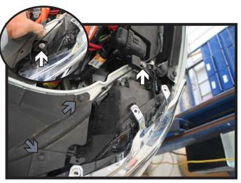
On the top side of the fascia, remove the two (2) push pins (gray). Then using a T25 Torx remove the two (2) screws from the headlight assembly (white). The second screw is underneath the cover (inset).
