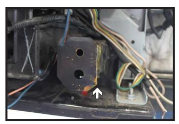
7. Using a reciprocating saw, trim off the outer edge of the extension flange flush with the weld for baseplate clearance. Do this on both sides of the vehicle.
