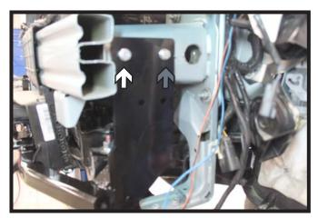
13. Install a 3/8" nut plate onto the rear bolt on the inside of the frame (gray). Do this on both sides of the vehicle. Fully tighten both bolts.
