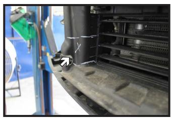
Trim the radiator shrouding approximately as shown for baseplate clearance. Do this on both sides of the vehicle.
