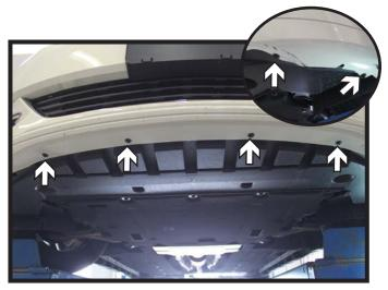
4. Using a 7MM socket, remove the eight (8) screws from the underside of the fascia. There are two (2) on each side and four in the middle.
