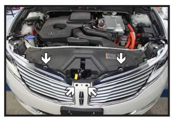
Using a T25 Torx, remove the four (4) screws from the top edge of the fascia.
