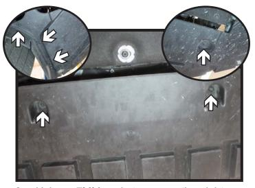
Using a 7MM socket, remove the eight
