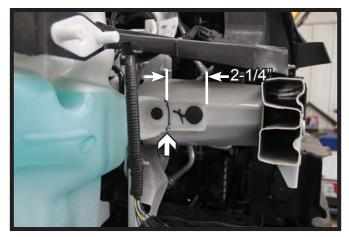
5. Using a utility knife, trim the outer flange of the washer fluid reservoir back approximately 2-1/4" as shown.
