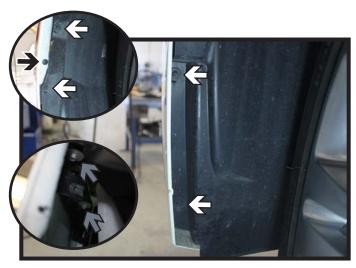
3. In the wheel well, using a 7MM socket, remove the four (4) screws (white). Then using a Phillips screwdriver remove the outer screw (black).
