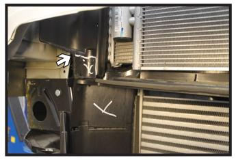
Trim the upper section of shielding just below the bumper and disconnect the lower section. Do this on both sides of the vehicle.
