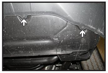
Using a 10MM socket, remove the four (4) screws from the underside of the fascia. There are two (2) on each side.
