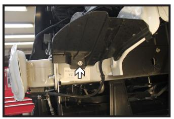
On the driver side, using a 10MM socket, remove the screw from the plastic shield. The shield will not be reinstalled.
