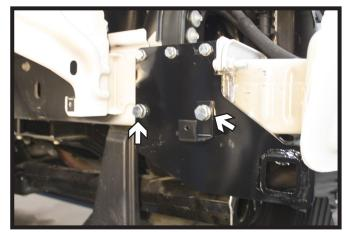
16. Using a 1/2" drill bit, drill the lower two (2) holes thru the frame wall. Install 1/2" bolts with lock washers into the holes with 1/2" nut plates on the inside of the frame. Do this on both sides of the vehicle. Fully tighten all hardware.
