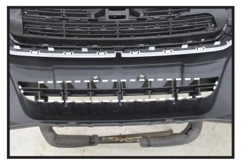
19. On the backside of the fascia, trim inside grill section out of the lower opening so it is one large opening.
