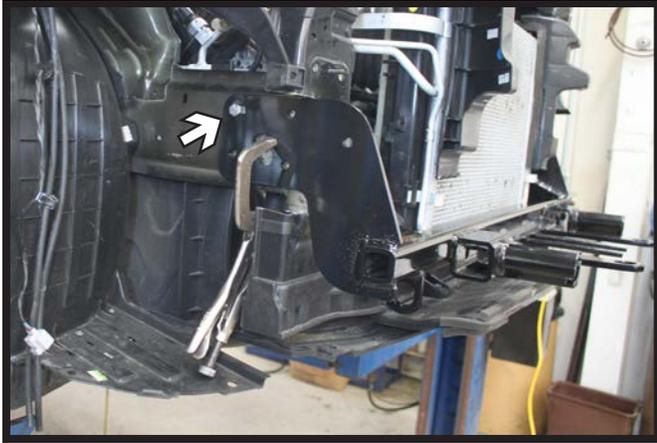
13. Using a 13/32" drill bit, drill the top back hole thru the frame. Install a 3/8"-16 x 1" bolt with lock washer into the hole and a 3/8" nut plate on the inside of the frame. Do this on both sides of the vehicle. Fully tighten all hardware.
