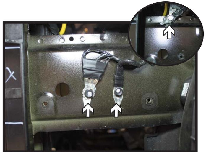
8. Using a 10MM socket, remove the two (2) ground wire screws from the side of the frame.
