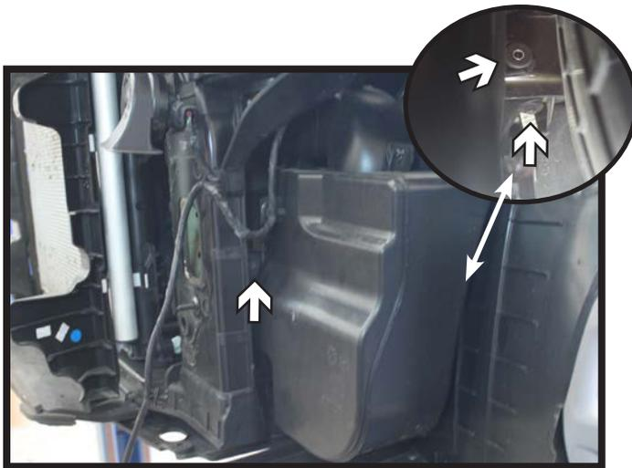
7. Using a 10MM socket, remove the three (3) screws from the air baffle. There are two (2) on the backside (inset) and one (1) in front. Disconnect the baffle and set aside.
