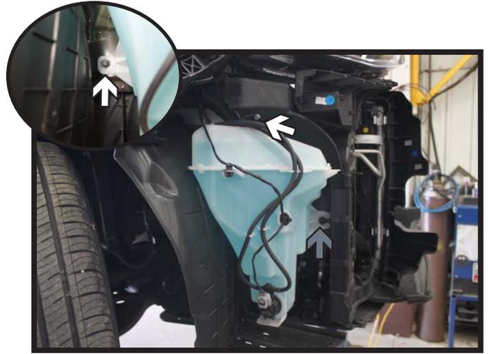
6. Using a 10MM socket, remove the two (2) screws from the washer reservoir (white). Then using a phillips screwdriver, remove the screw from the front of the washer reservoir (gray). Disconnect/plug all lines and set reservoir aside.
