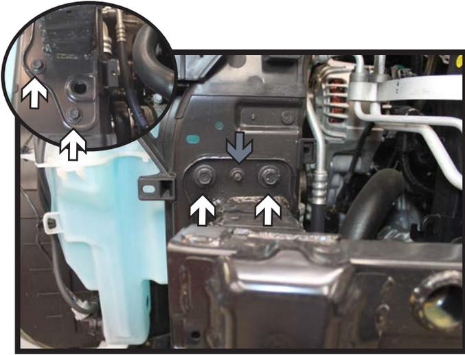
5. Using a 12MM socket, remove the four (4) screws from the bumper (white). Then using a 10MM socket, remove the nut (gray). Do this on both sides of the vehicle. Set the bumper aside.
