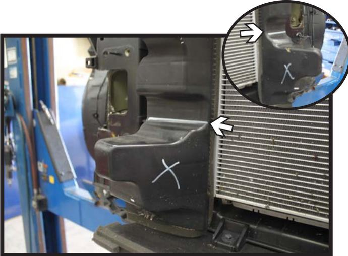
11. Trim off the lower sections of the plastic shrouding as shown on both sides of the vehicle for baseplate clearance.
