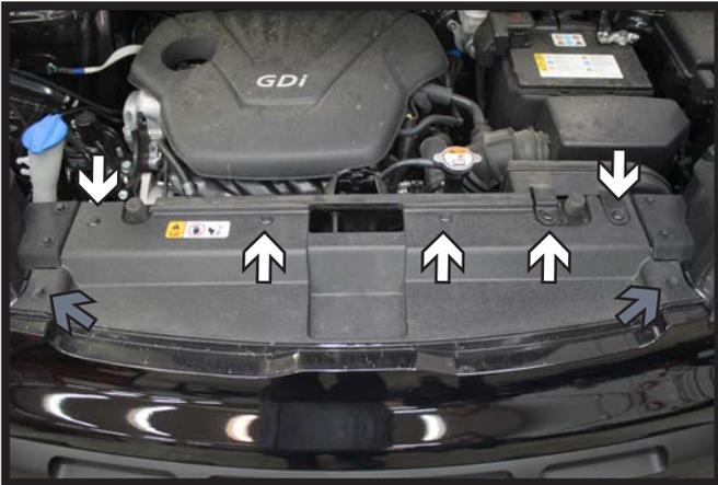
1. Using a 10MM socket, remove the two (2) screws from the top edge of the fascia (gray). Then remove the five (5) push pins (white).
