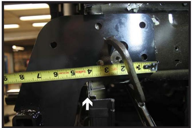
12. Position the baseplate onto the vehicle. Set the backside 4-1/4" from the face of the frame, level and clamp into position.
