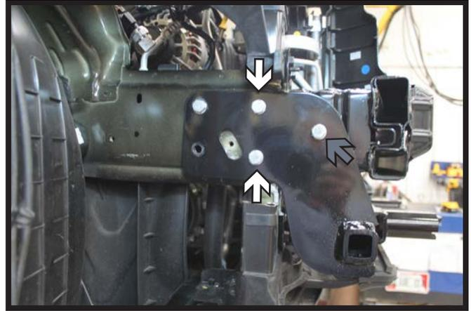
14. Install a 3/8"-16 x 1" bolts with lock washers into the holes and a 3/8" nut plates on the inside of the frame. Do this on both sides of the vehicle. Fully tighten all hardware.
