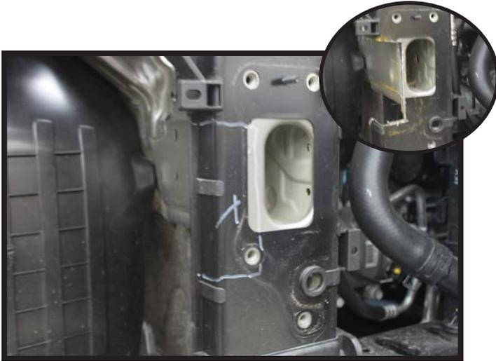
9. Using a reciprocating saw, remove the area just below the knob down just below the factory hole and back flush to the side of the frame. Do this on both sides of the vehicle.
