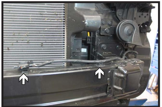
4. Disconnect the temperature sensor from the top side of the bumper and set aside.
