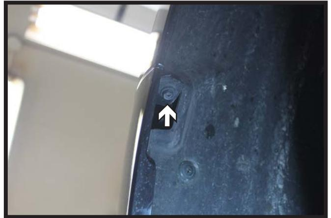
2. Using a 8MM socket, remove the screw from the top edge of the wheel well. Do this on both sides of the vehicle.
