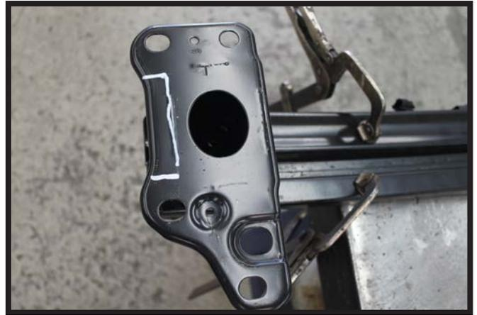
10. Temporarily reinstall the bumper and trace the backside along the frame cuts on both sides. Remove the bumper and trim the marked areas with a reciprocating saw.
