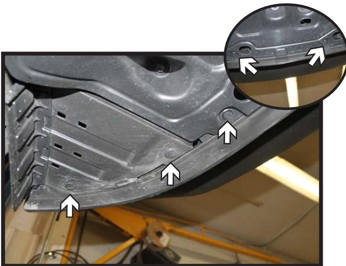
3. Remove the eight (8) push pins from the underside of the fascia. There are three (3) on each side and two (2) in the middle. Remove the fascia from the vehicle, disconnecting any electrical connections and set aside.
