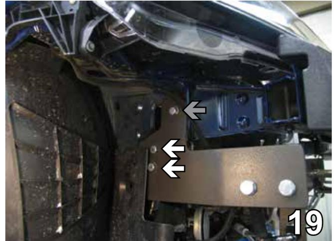
19. On the passenger side, using the baseplate as a template, drill all three holes with the 13/32" drill bit. Insert into the bottom two holes (white arrows) 3/8" x 1 1/4" hex bolts with Loctite Red, tighten with 3/8" lock washers and 3/8" hex nuts. Insert a 2" hex bolt with 3/8" lock washer using Loctite Red into the top hole (gray arrow) and tighten with 1" nut plate. Tighten the baseplate to the end plates.
