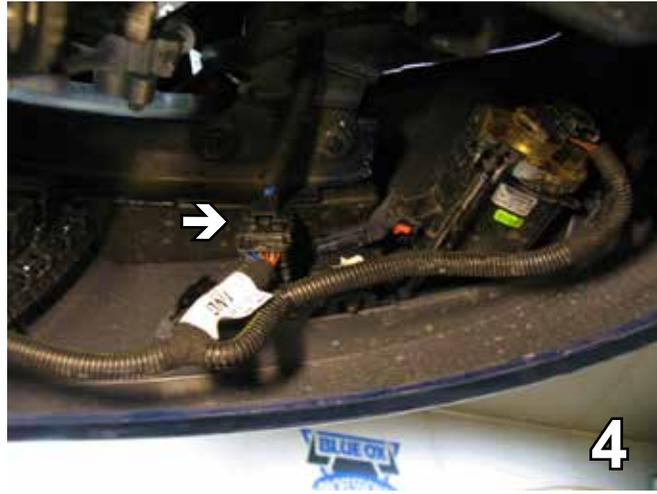
4. On the passenger side only, up in behind the front tire, unplug the master connector.
