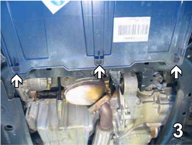
3. Remove three push pins from underneath on the bottom edge of the belly pan. Set the push pins aside to be reinstalled later.
