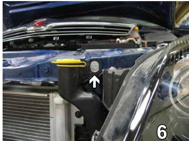
6. Using the 10MM socket, remove the top metric bolt from the washer reservoir. Set the bolt aside to be reinstalled later.
