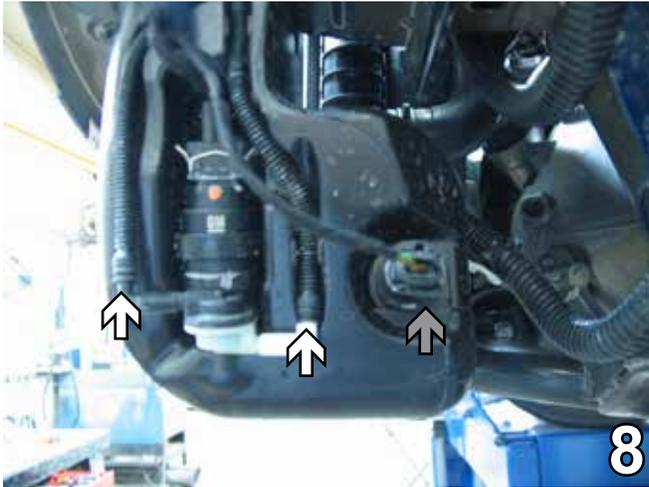
8. Pull the three washer reservoir hoses out. Disconnect two (white arrows) and plug their ends. Unplug the electrical connection (gray arrow). Set the washer reservoir aside to be reinstalled later.
