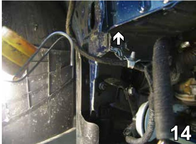
14. Cut straight across under the horn, making sure to be level. Do this on both sides.
