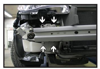
7. Remove the metal bumper, using a 12MM socket, remove the four (4) bolts from the bumper. Do this on both sides of the vehicle.
