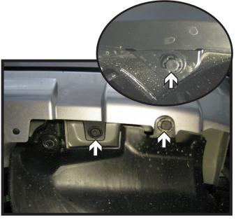
4. Using a flat screwdriver, remove six (6) push pins from the underside of the fascia. There is one (1) in front of the tire and two (2) in the towards the middle. Do this on both sides of the vehicle. Pull fascia corners outwards, then pull fascia forward to remove.
