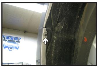
2. Just forward the front tire, push the pin in the center to release. Do this to both sides of the vehicle.
