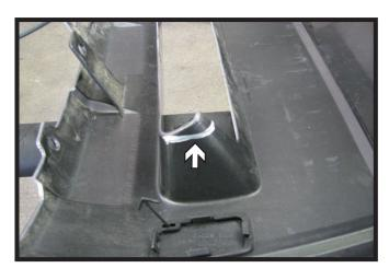
19. Hold the fascia as close to it's original position and mark the backside of the fascia, trim as needed. Reinstall the fascia.
