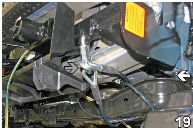
18. Start 3/8"-16 x 1-1/2" bolts in top hole (white arrow) with lock washers and attach to 3/8"16 nut plates. Insert 3/8"-16 x 2" bolts in the bottom hole (gray arrow) attach to a spacer and 3/8"-16 nut plate inserted into the end of the frame rail. Use Loctite on all bolts before tightening.
