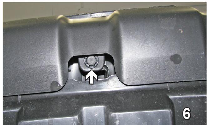
5. Remove the push pin from the tab on the lower edge of the fascia. Do this on both sides. Set push pins aside for later reinstallation.
