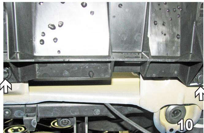
10. Underneath the cover in order to remove the air dam, remove three (3) push pins. One on each side and one in the middle. Set the push pins aside for later reinstallation.
