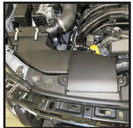
24. Reinstall windshield washer reservoir, horn, filter and sub-tank, and cover.
