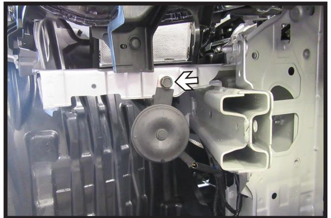
13. Using a 12MM socket remove the one (1) bolt holding the horn on the passenger side of the vehicle. Remove and set aside to be reinstalled later.
