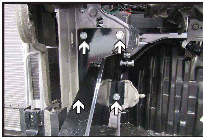
19. Insert the four (4) 8MM bolts with flat washer and lock washer into the front of the baseplate. Do this on both sides of the vehicle.
