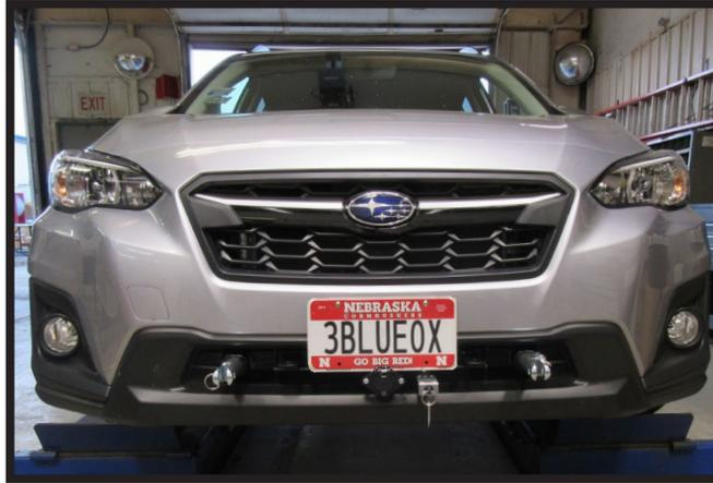
25. Hold the fascia as close to its original position, mark and trim the fascia around the convenience links and attachment tabs. Reinstall the fascia and fascia cover.
