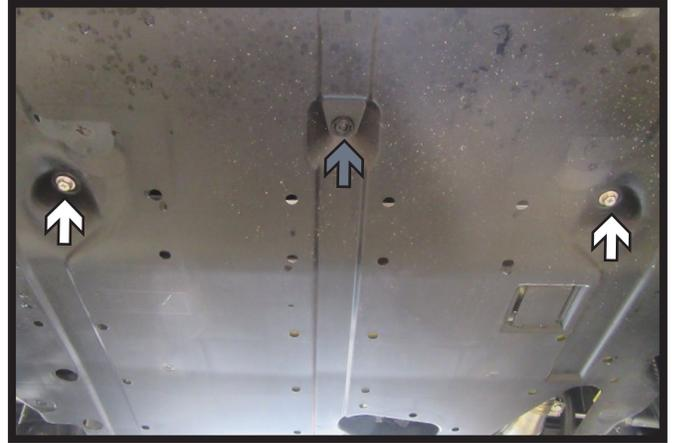
15. Using a 12MM socket remove the two (2) bolts (white) from the belly pan of the vehicle. Then remove the one (1) push pin (gray). The belly pan will hang loose once these are removed.
