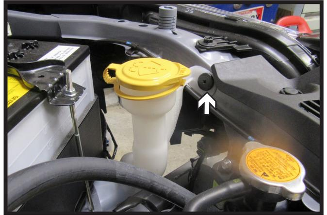
8. Using a Phillips screw driver remove the plastic screw from the top of the windshield washer reservoir on the driver side of the vehicle.
