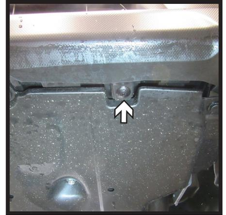
4. Using a Phillips screw driver remove the three (3) plastic screws from the underside of the fascia.
