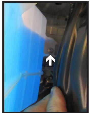
9. Unplug all of the fluid lines from the windshield washer reservoir. Then using a 10MM socket, remove the three (3) bolts holding the reservoir in place. Remove and set aside to be reinstalled later.
