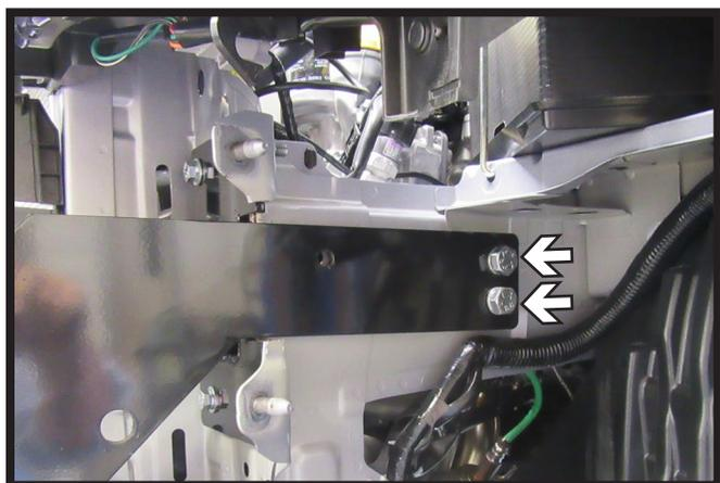
20. Remove the two (2) bolts on the side of the baseplate, one at a time. Apply Loctite® Red and tighten to appropriate torque. Do this on both sides of the vehicle.
