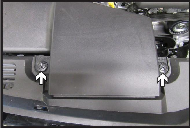
10. Using a flat head screw driver turn top two (2) screws 1/4 of a turn and remove plastic piece from the passenger side of the vehicle, to be reinstalled later.
