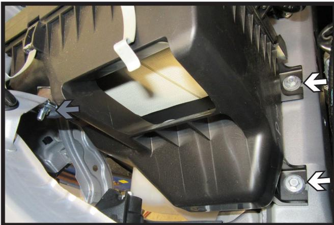
12. Using a 10MM socket remove the two (2) bolts (white) and one (1) nut (gray) as indicated from the passenger side of the vehicle. Remove air filter and sub tank and set aside to be reinstalled later.
