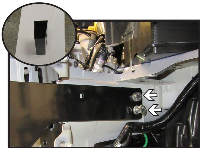
18. Slide the baseplate onto the frame. Insert wedge piece (inset) between the frame and the baseplate with the narrow edge towards the front and the wide edge towards the back. Once the wedge is in place start the two (2) 12MM bolts with lock washers. Tighten but do not use Loctite® Red at this time. Do this on both sides of the vehicle.
