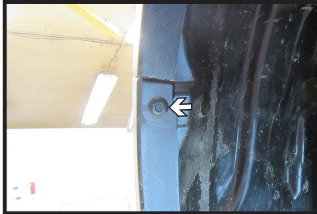
2. Remove the one (1) push pin from inside of the wheel well by pressing on the center. Do this on both sides of the vehicle.
