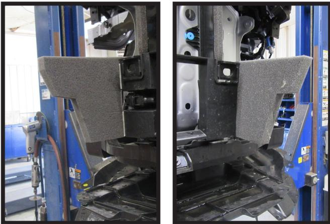
16. Remove the foam pieces from each side on the front of the vehicle.
