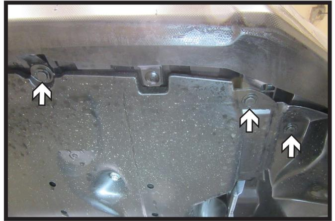
3. Remove five (5) push pins from the underside of the fascia. Do this on both sides of the vehicle.
