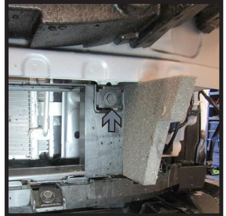
6. Using a 12MM socket, remove the four (4) bolts (white) from the bumper as indicated. Then using a 10MM socket remove the one (1) bolt (gray). Do this on both sides of the vehicle. Remove bumper, it will not be reinstalled later.
