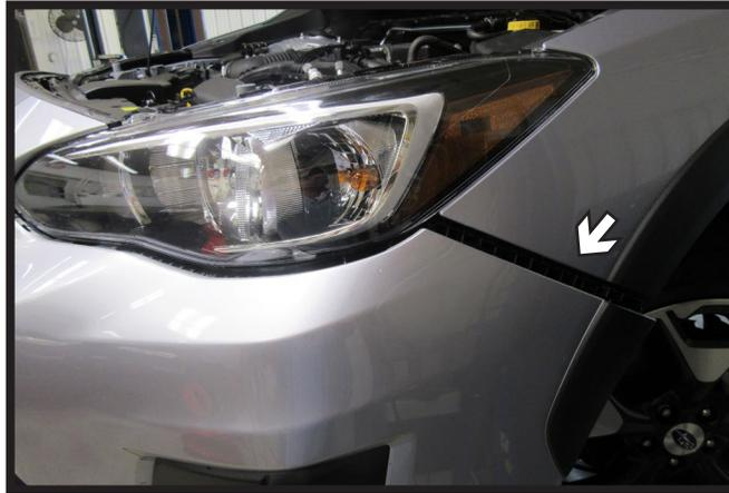
5. Grasp the fascia near the headlight and pull upward and outward to remove. Set aside to be reinstalled later.
