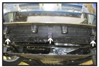
9. Using a 10MM socket remove the three (3) bolts from the plastic piece at the bottom of the grill and remove piece. Set aside to be reinstalled later.
