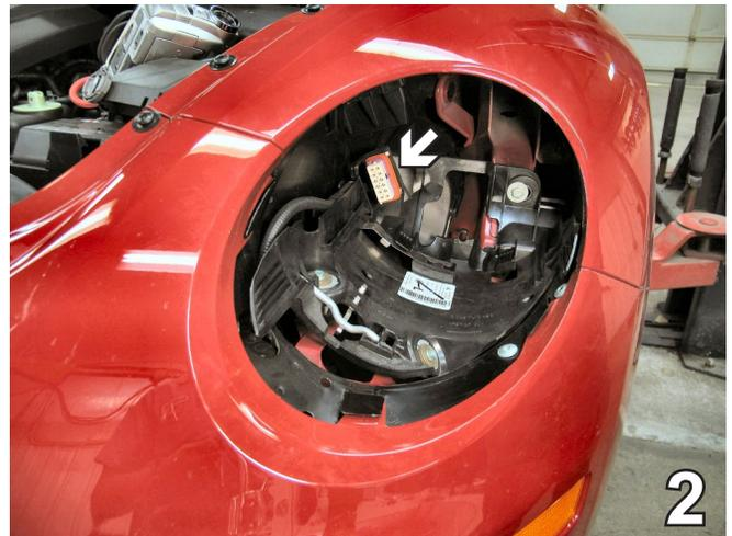
2. On the driver's side, push down on a silver clip found behind the battery box and headlight housing. It can only be reached from above, so a long tool such as a screwdriver is needed to reach it. With the clip pressed down, pull headlight assembly forward to remove. A firm tug may be needed to release the headlight assembly from the electrical plug (see the white arrow in the photo above). Do this to both sides of the vehicle. Set headlight assemblies aside to reinstall later.
