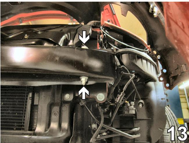
13. Remove the metric hex nut on the bottom of the metal bumper, using the 18MM socket and wrench, remove the metric bolt. Do this to both sides of the metal bumper. Remove metal bumper by pulling forward. Set bolts, hex nuts and bumper aside to be reinstalled later.
