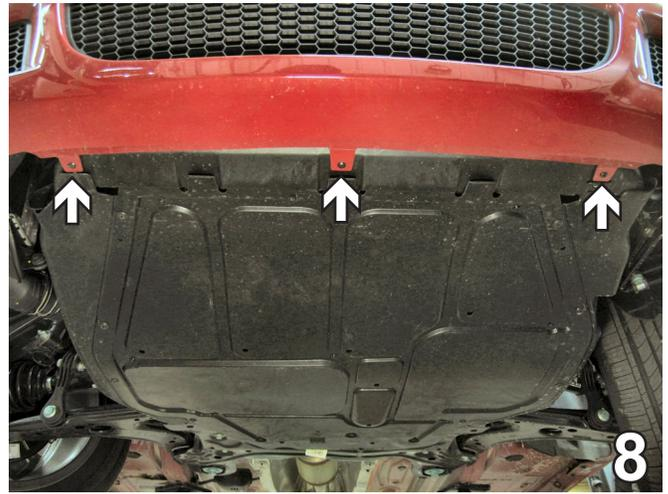
8. Use a small flat screwdriver to remove three push pins on the lower side of the fascia. See next step for removal technique.
