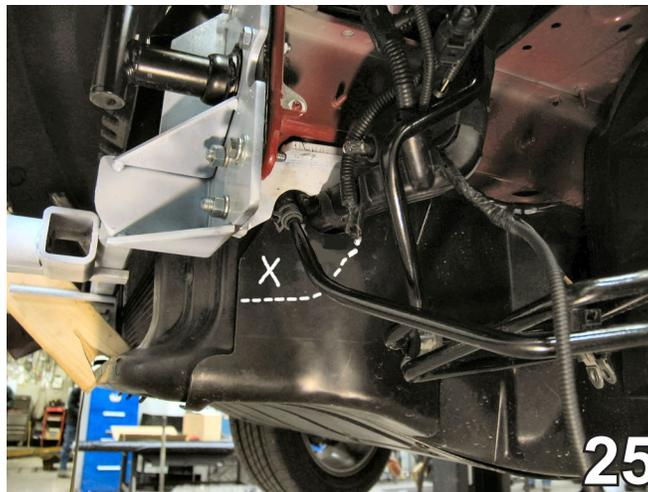
25. On the driver's side, mark and trim an area just below the wiring harness. Doing this allows the wiring harness to be moved while drilling. Avoid cutting the wire harness when using the utility knife.
