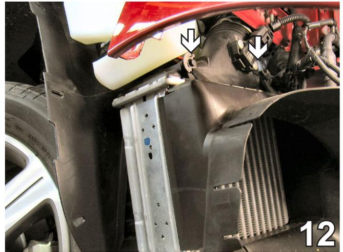
12. Lift the fascia up, disconnect marker lights and temperature sensor (if the vehicle is equipped with such features). Use a 1" x 4" x 22" block of wood (not provided) as a brace to prop up the fascia. Remove the air dam shield immediately in front of the turbo cooler (if equipped on vehicle) simply by pulling it forward. Doing this releases it from two clips. Set air dam shield aside to reinstall later.
