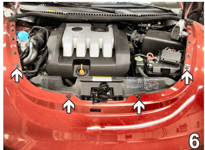
6. Using a T30 Torx socket, remove four metric bolts from the top side of the fascia. Set bolts aside to reinstall later.
