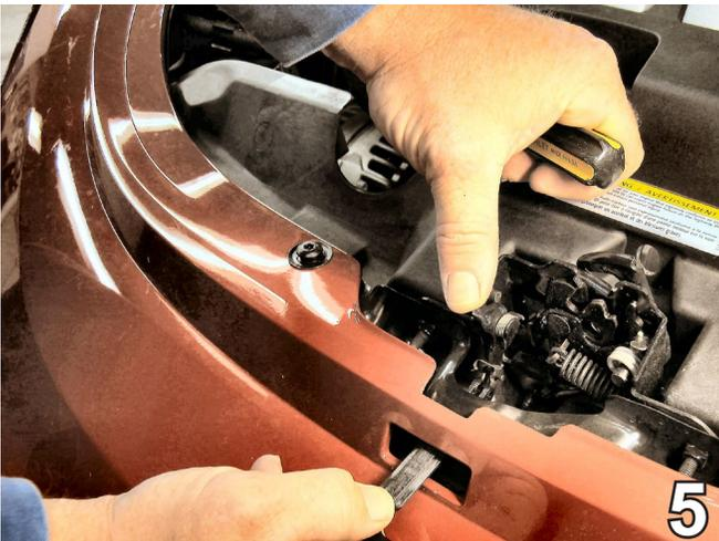
5. Move hood release handle upwards and carefully guide the hood release out. Pay special attention to not allow the clip to fall out while guiding the hood release out. Set hood release handle aside to reinstall later.
