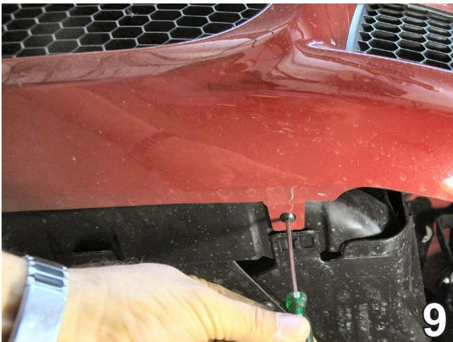
9. Using the small flat screwdriver, push up on the center of pushpin. The pushpin is released. Do **NOT** push center push pin all the way through the base. Pry the pushpin out with the screwdriver. Set push pins aside to reinstall later.
