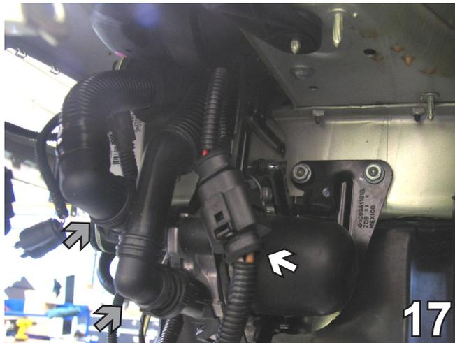
17. On the driver's side, disconnect the electrical connection to the coolant fan (see white arrow). Disconnect the two air lines (see grey arrows) by squeezing the sides of their lower ends to release clips.
