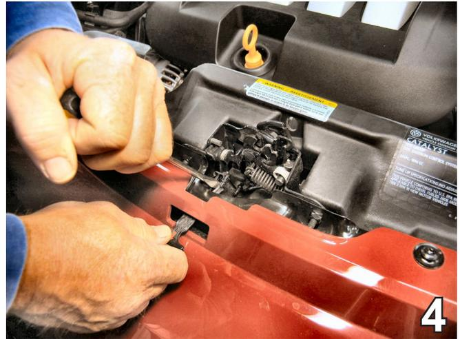
4. Insert and twist a flat screwdriver to separate the hood release handle from the pins securing it.
