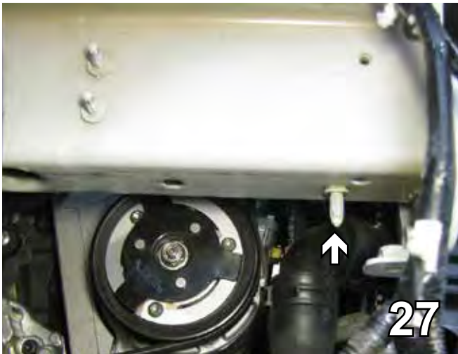
27. On the passenger side on the bottom of the frame, use a pliers to wiggle the stud off.
