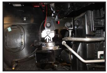
4. Using a 5/16" Allen socket or wrench, remove the screw from the horn bracket and set the horn assembly aside. Do this on both sides of the vehicle.
