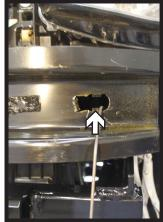
13. Using a 1-1/4" hole saw, drill an access hole on the underside of the bumper on the passenger side only (left).Using a reciprocating saw, enlarge the existing hole on the driver side of the bumper (right).
