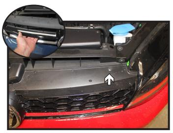
Using a T25 Torx, remove the two (2) screws from the top edge of the grille.
