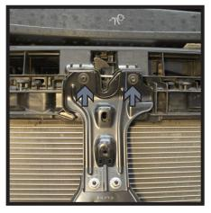
Using a 16MM socket, remove the eight (8) bolts from the bumper. There are four (4) on each side, two (2) on top & two (2) on bottom (white).
