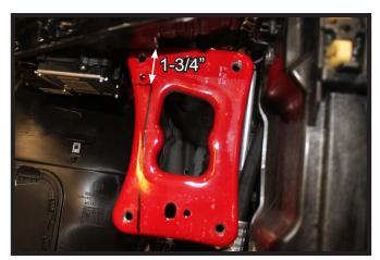
9. Using a reciprocating saw, trim the outer flange of the frame down 1-3/4" from the top and back to the face of the frame down thru the bottom lip. Do this on both sides of the vehicle.
