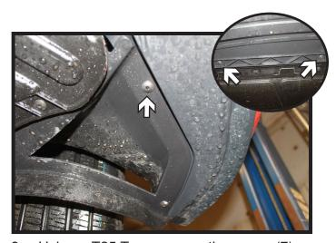
3. Using a T25 Torx, remove the seven (7) screws from the underside of the fascia. There are two (2) on each side in each corner and three (3) across the middle. Remove the fascia from the vehicle, disconnecting any electrical connections and set aside.
