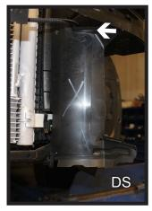
12. Trim the plastic shielding off just below the bumper on both sides of the vehicle. The shielding is not reinstalled.
