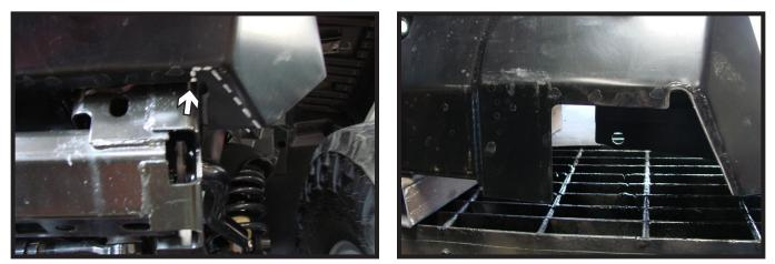
7. **ARB Stubby Bumper Only:** Mark the under side of the bumper as shown (left). Using a reciprocating saw trim the under side of the bumper to clear the baseplate (right). Do this on both sides of the bumper.
