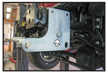
4. Position the baseplate onto the vehicle. Level and clamp the baseplate securely. Install a 5/8"-11 x 1-1/2" bolt with lock washer into the lower hole and a 5/8" whiz nut on the inside of the frame. Do this to both sides of the vehicle. Fully tighten all hardware.
