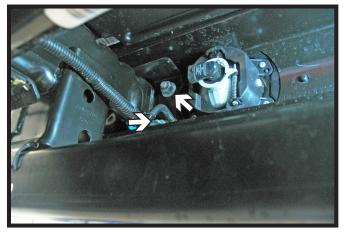
3. Using a 18MM socket, remove the two (2) bolts on inside edge of frame. Do this to both sides of the vehicle.
