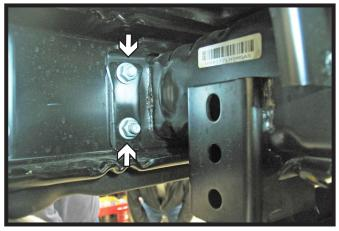
2. Using a 18MM socket, remove the two (2) bolts along the outside edge of frame. Do this to both sides of vehicle.
