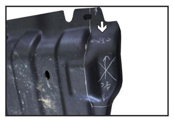
6. Trim the belly pan as shown. Using a reciprocating saw, cut 2-1/2" inward and downward 7-3/4" to allow proper clearance for the baseplate.
