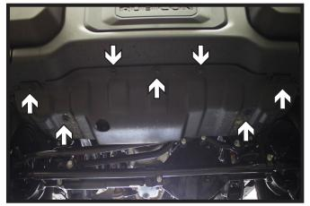
Using a 15MM socket, remove the seven (7) bolts from the bottom of the belly pan. There are two (2) on each side and three (3) across the center. Set the pan aside.
