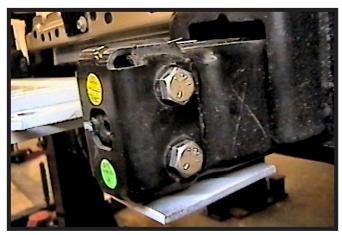
9. Hold up the baseplate up and align with the existing tow hook holes. Insert 1/2"-13 x 3-1/2" bolts into the holes. Be sure that baseplate is level with the vehicle and temporarily tighten with a nut.
