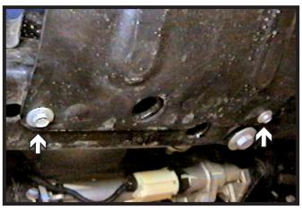
5. Remove the four (4) bolts from the belly pan using the 13MM socket, pull the belly pan down to remove. Set the belly pan aside.
