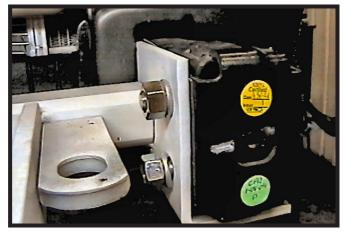
12. Remove the four (4) hex nuts from the 1/2" x 3-1/2" bolts. Install lock washers and fully tighten all fasteners.
