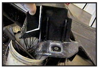
Reinstall the metal bumper. Trim the belly pan as shown above, then reinstall. Reinstall the grille and plug in all electrical connections.
