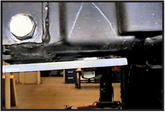
10. Using the baseplate template, drill the lower hole into the frame with the 17/32" drill bit. Do this to both sides of the vehicle. Loosen bolts installed in Step 9, slide the 1/2" flat washer between the frame and the baseplate to align with the drilled hole.
