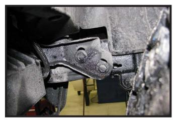
7. Using the 15MM socket, remove two (2) bolts from the bumper bracket, pull the bumper forward and unplug the electrical lines. Set the metal bumper aside.
