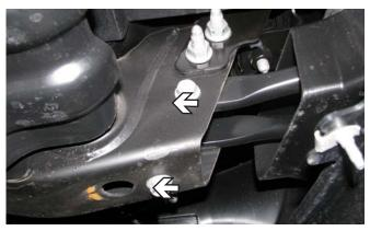
7. Using the 18MM socket, remove the two metric bolts from the top and side of the tow hook. Do this to both sides of the vehicle.
